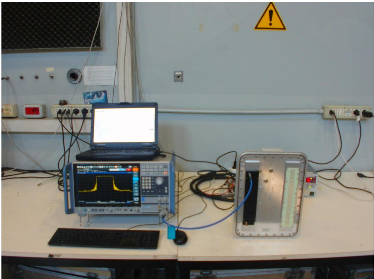
**1.4 Frequency stability test set-up**
