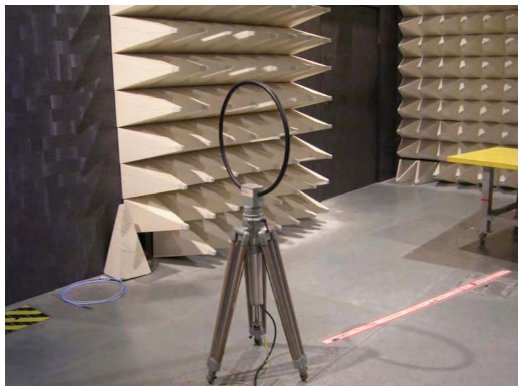
For radiated emissions 9kHz-1GHz
