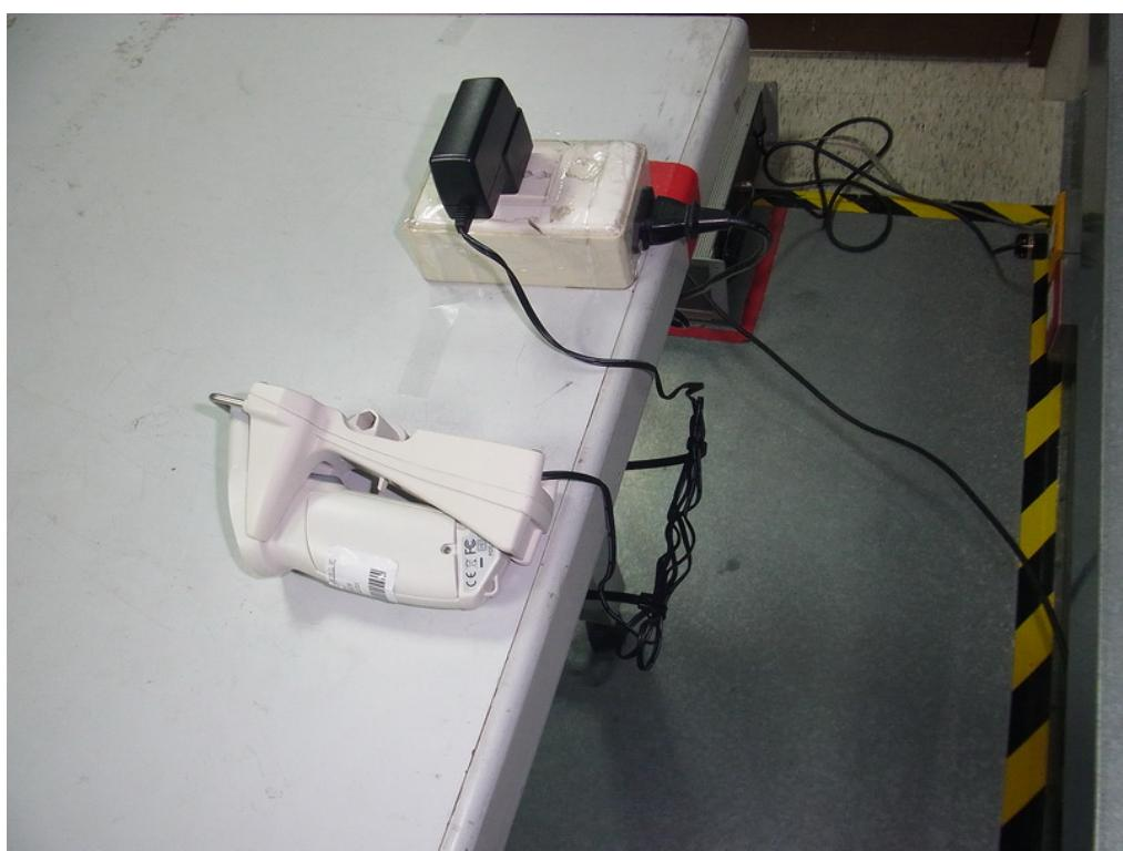
**Radiated spurious emission test photos****9K-30MHz**
