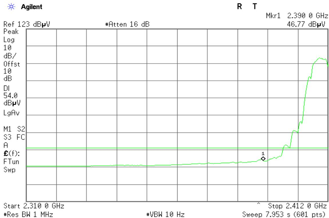
**Band Edges (IEEE 802.11b / CH High)****Detector mode: Peak****Polarity: Vertical**
