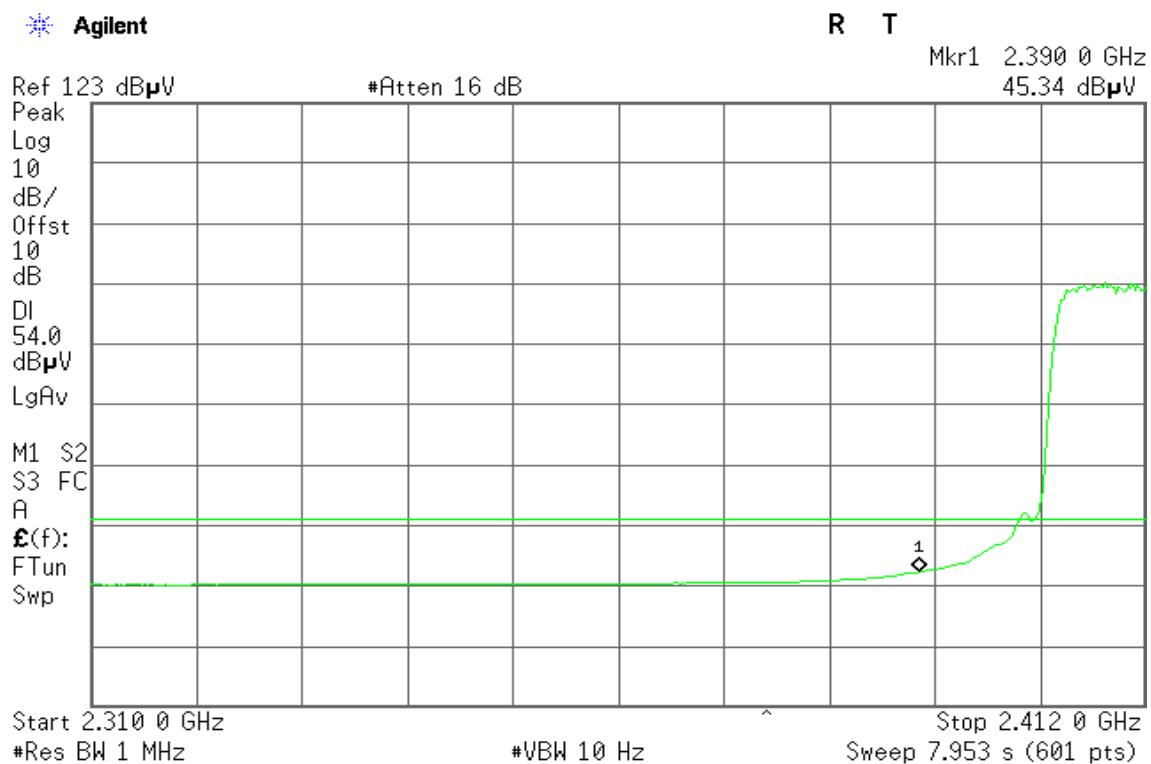
**Band Edges (IEEE 802.11g / CH High)****Detector mode: Peak****Polarity: Vertical**
