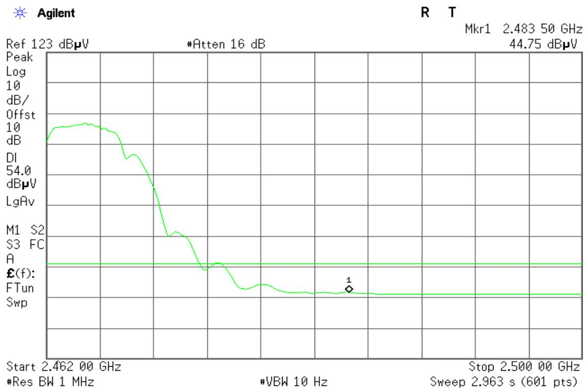
**Band Edges (IEEE 802.11g / CH Low)****Detector mode: Peak****Polarity: Vertical**
