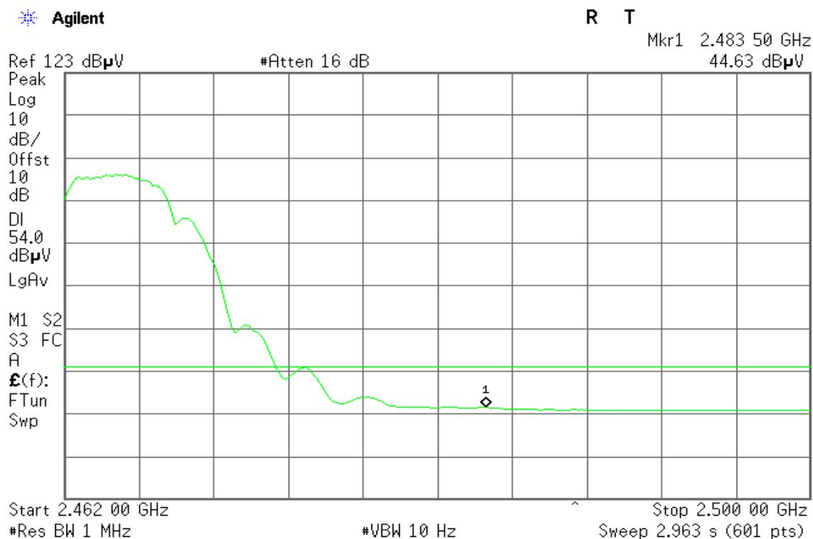
**Detector mode: Peak****Polarity: Horizontal**
