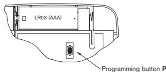
3. Press programming button P auf on the back of the device briefly. The shutter/blind will start to move up and down. This will happen for approximately 2 minutes.
