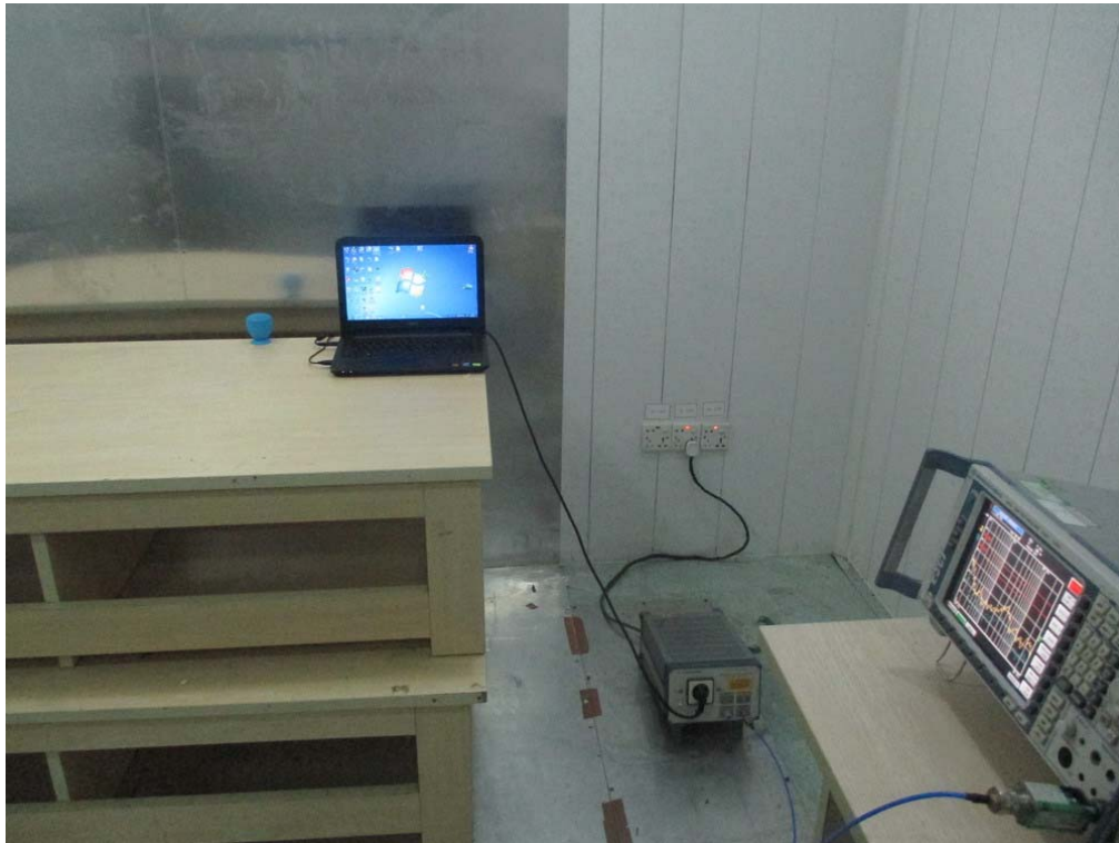
FCC RADIATED EMISSION TEST SETUP
