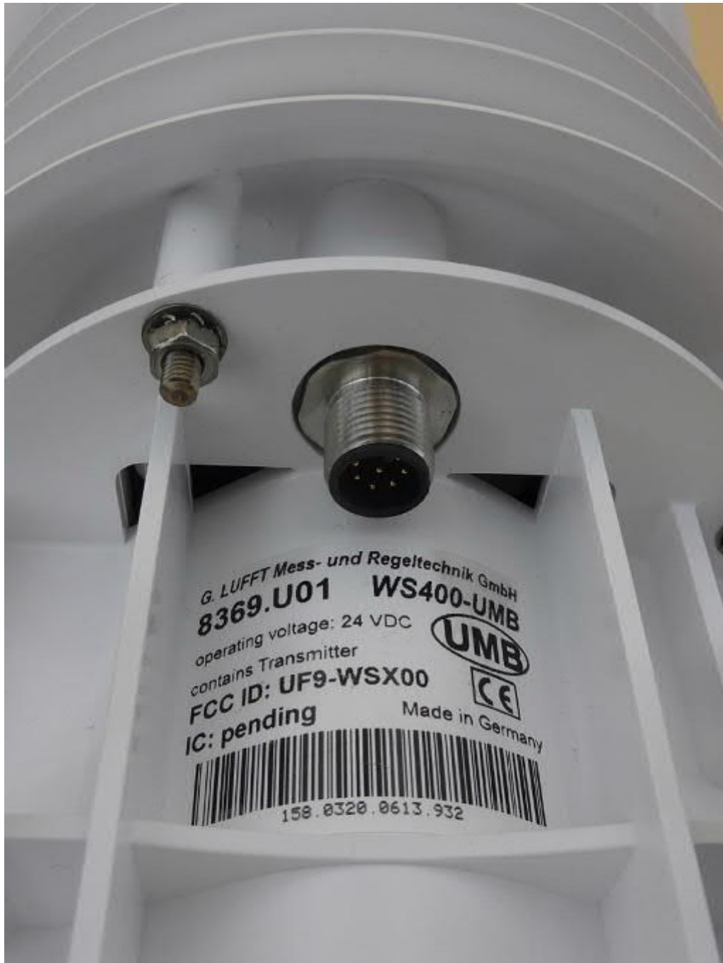
WS400-UMB, type plate and connector view
