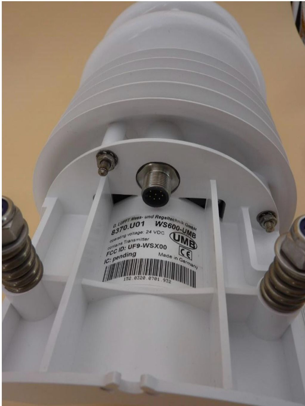
WS600-UMB, type plate and connector view
