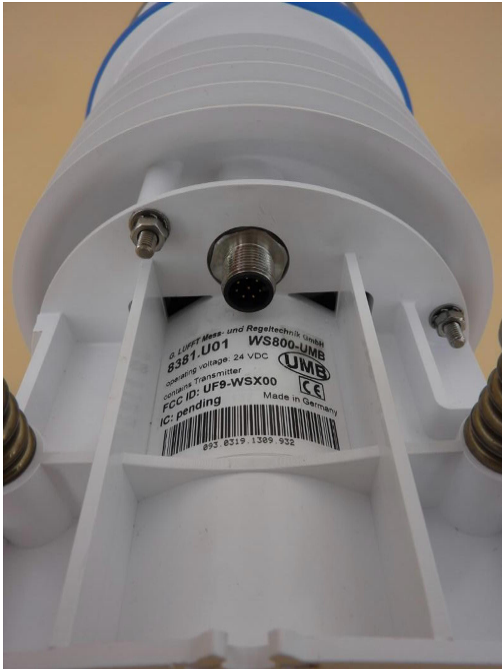
WS800-UMB, type plate and connector view
