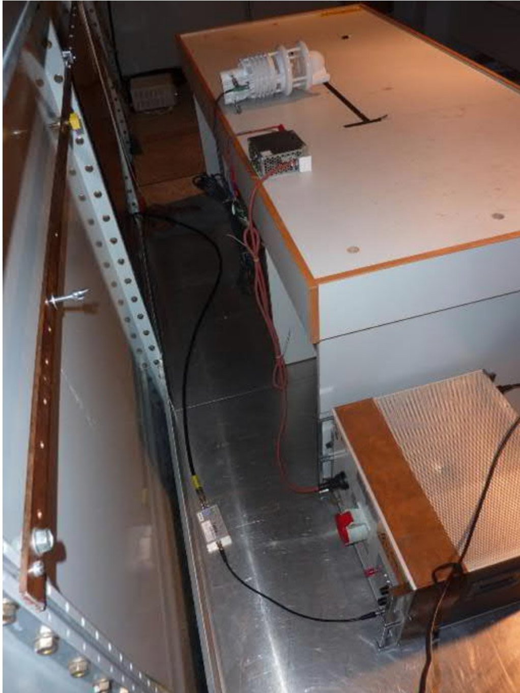
WS700-UMB, test setup shielded chamber
