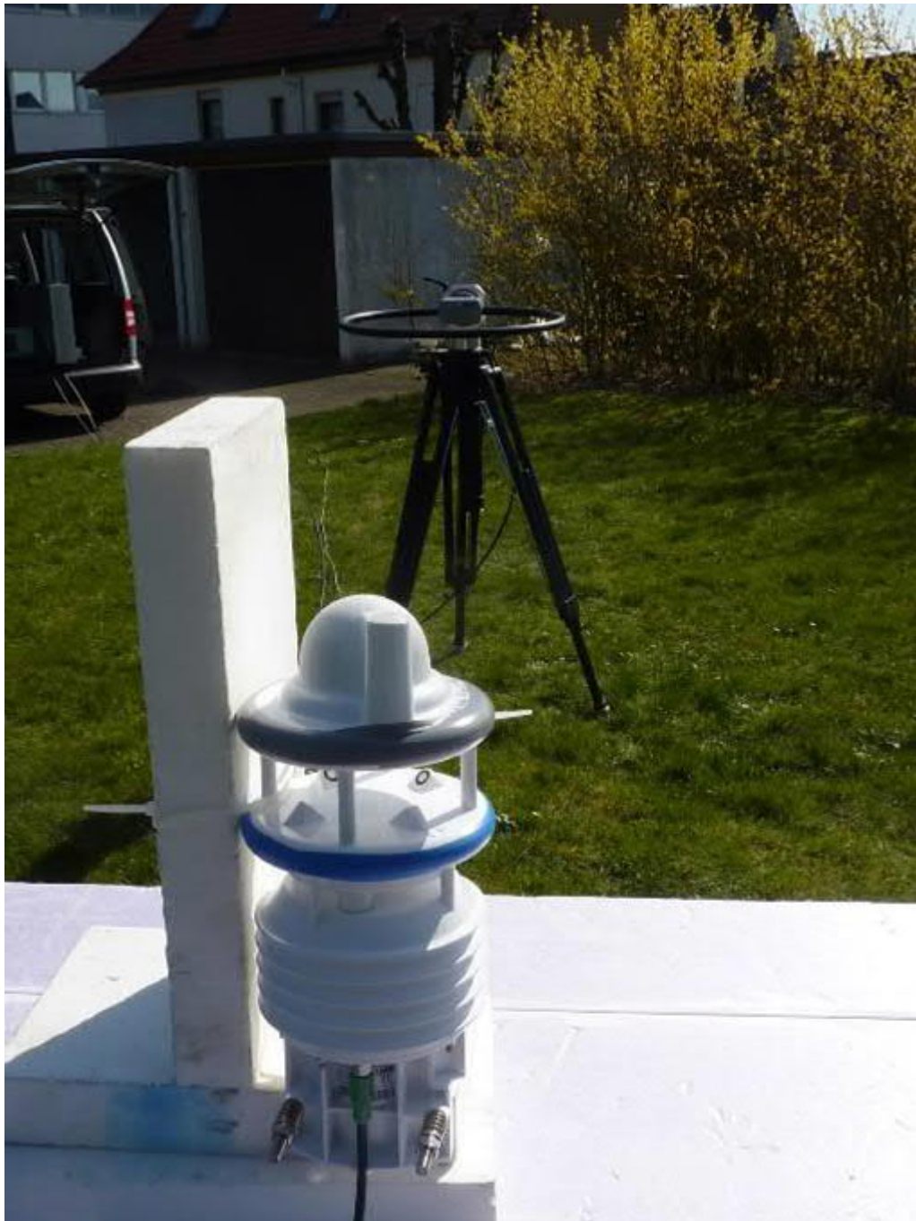
WS800-UMB, test setup outdoor test site
