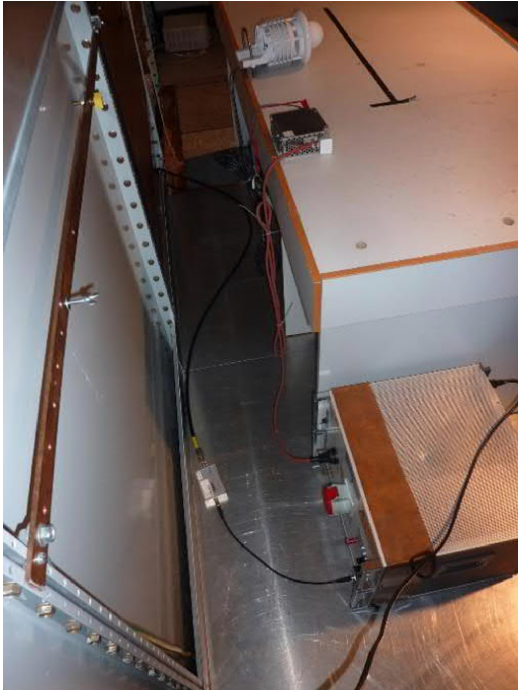
WS400-UMB, test setup shielded chamber
