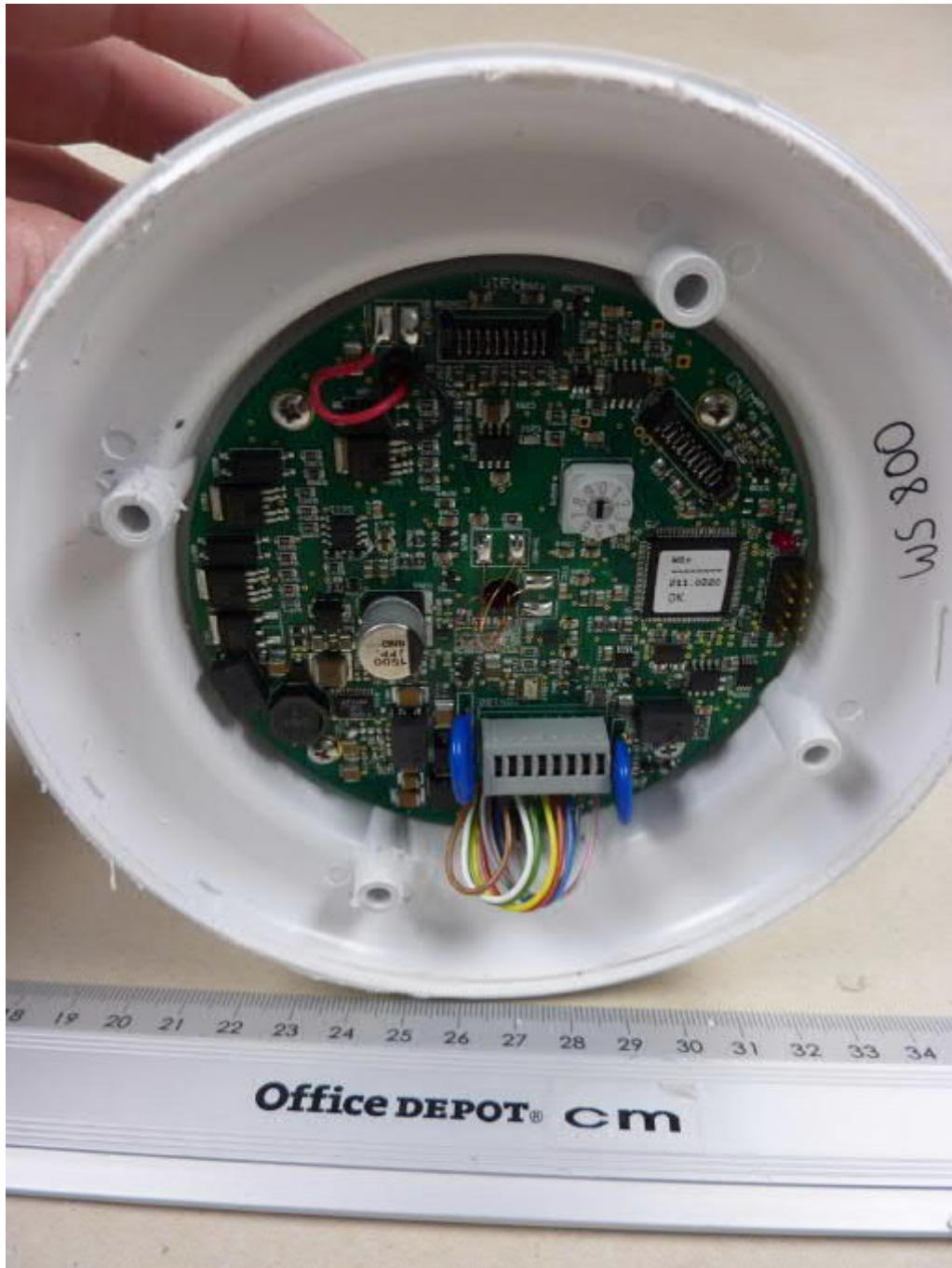
WS800-UMB housing with main PCB, shielding removed
