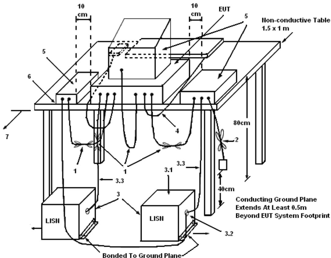
1. Interconnecting cables that hang closer than 40 cm to the ground plane shall be folded back and forth in the center forming a bundle 30 to 40 cm long.
