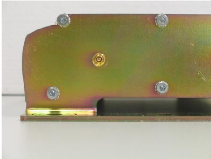
Figure 4: GPS antenna connector
