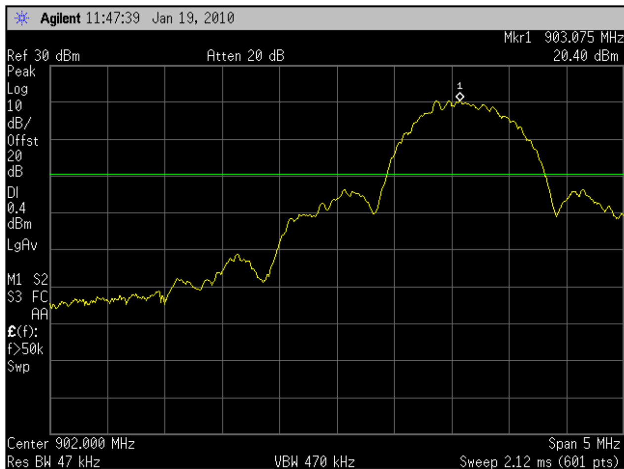
Plot 5-1: Lower Band Edge: Peak Measurement 903 MHz; 1000K SIN Modulation
