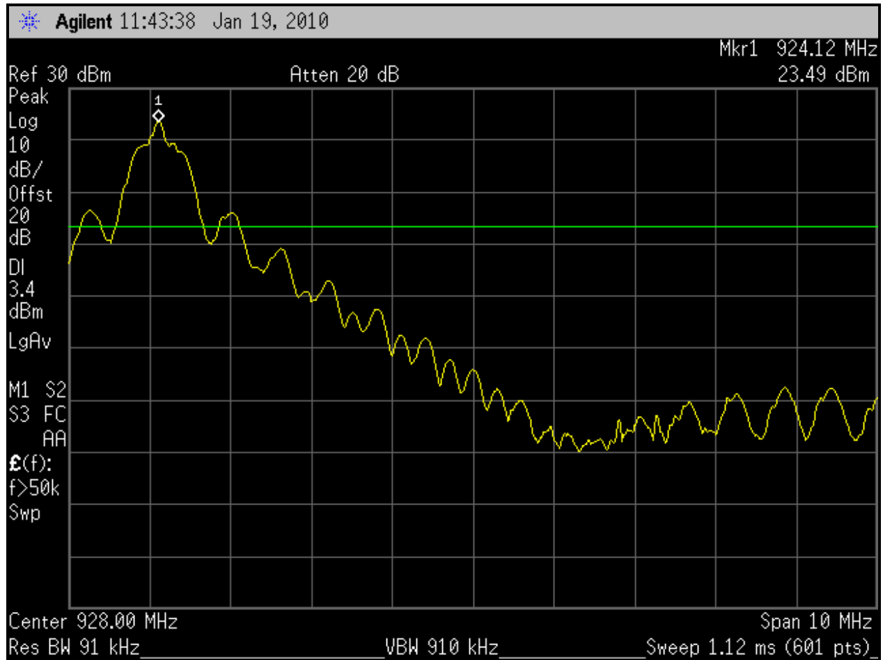
Plot 5-6: Upper Band Edge: Peak Measurement 924 MHz; BPSK40 Modulation
