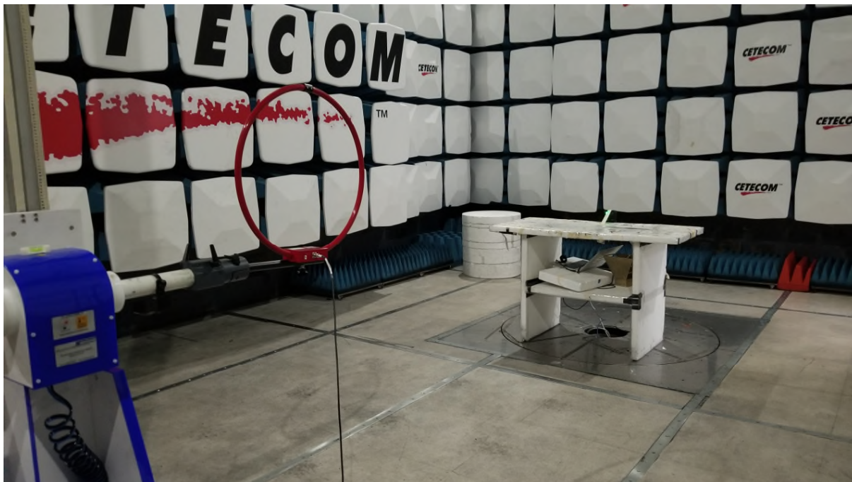
Photo 1: Emissions in frequency range 9 kHz to 30 MHz
