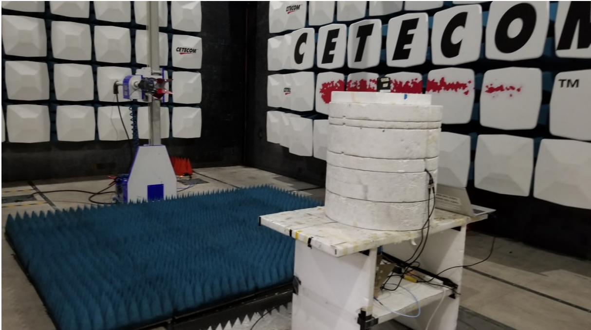
Photo 4: Emissions in frequency range 3-18 GHz
