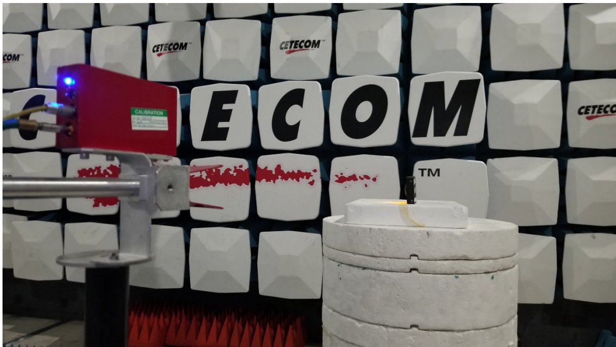
Photo 5: Emissions in frequency range 18-40 GHz
