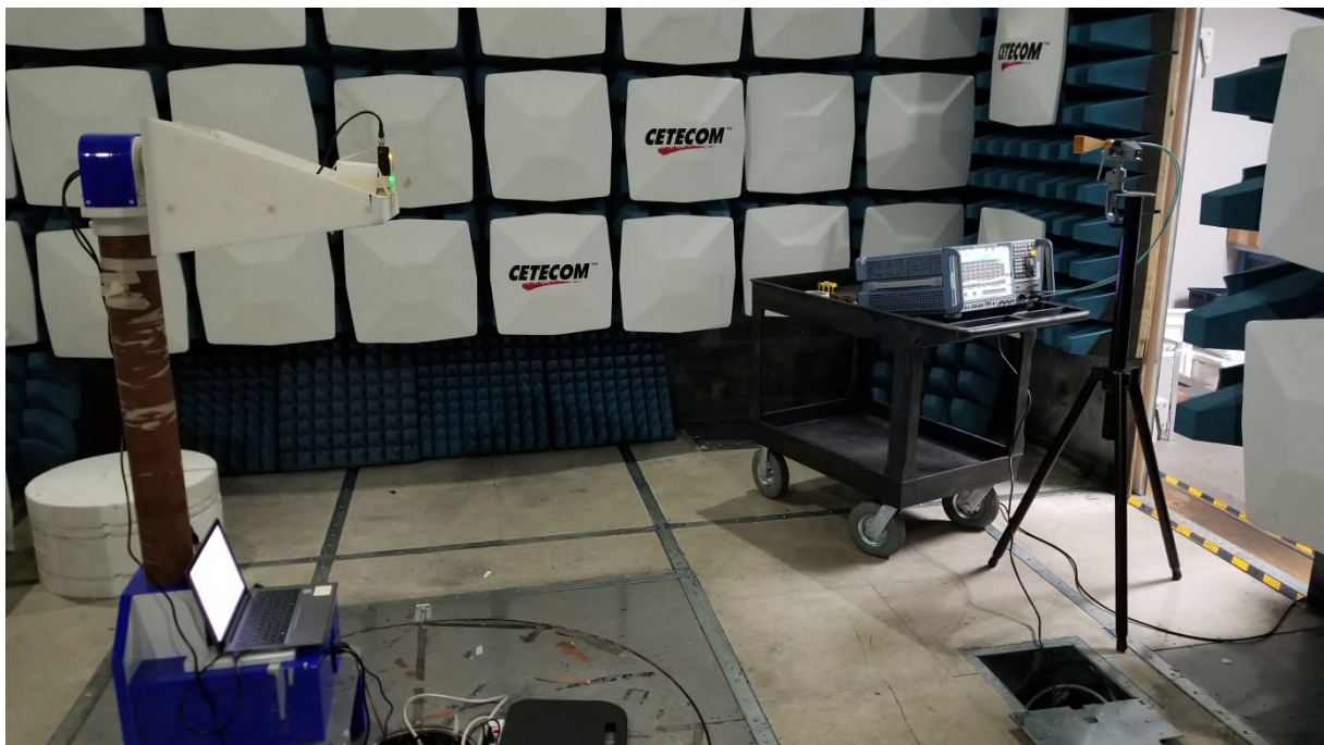
Photo 6: Emissions in frequency range 40-60 GHz (for other frequency ranges above 40 GHz, other external mixer and antenna are applied)
