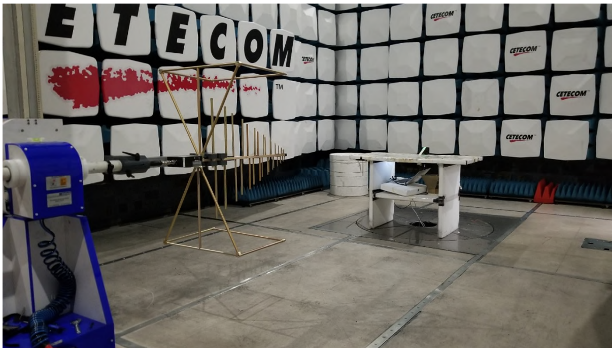
Photo 2: Emissions in frequency range 30 MHz to 1 GHz
