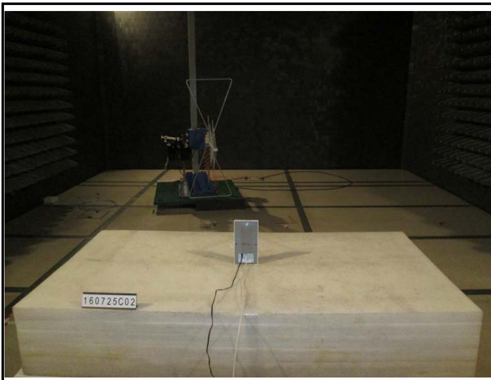
Radiated Emissions above 1 GHz Test
