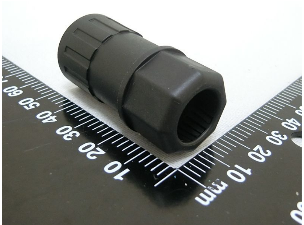
Waterproof Covering (Cable Gland) 1 used for EUT 1
