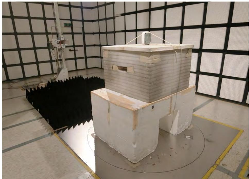
For Scanning Radio 3 – EUT in X axis
