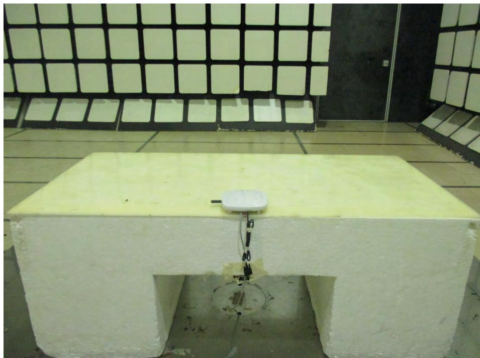
**Test Configuration: Above 1GHz / Test Mode: Mode 1, Mode 2 for bandedge, Mode 3**
