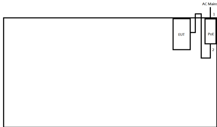
Test Setup Diagram – AC Line Conducted Emission Test (Group 1/Scanning Radio)
