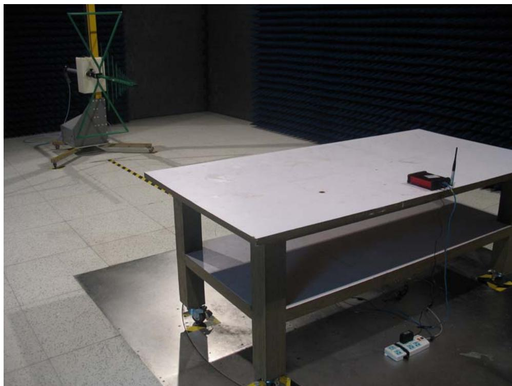
Test Mode : Mode 4: Transmit by 802.11g turbo g
