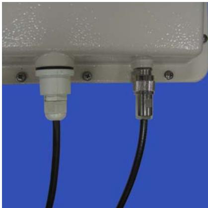
7. Connect the Access Point to the ground via ground connection which is beside the RJ-45 port.
