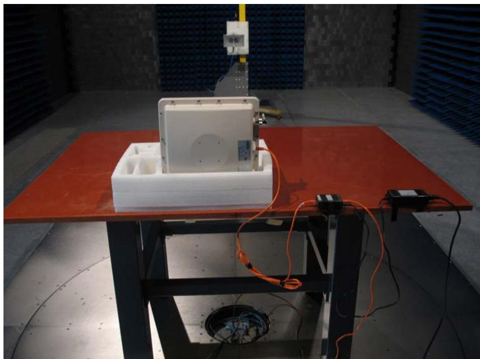
Test Mode: Mode4: Transmitter 802.11a with Inside Antenna
