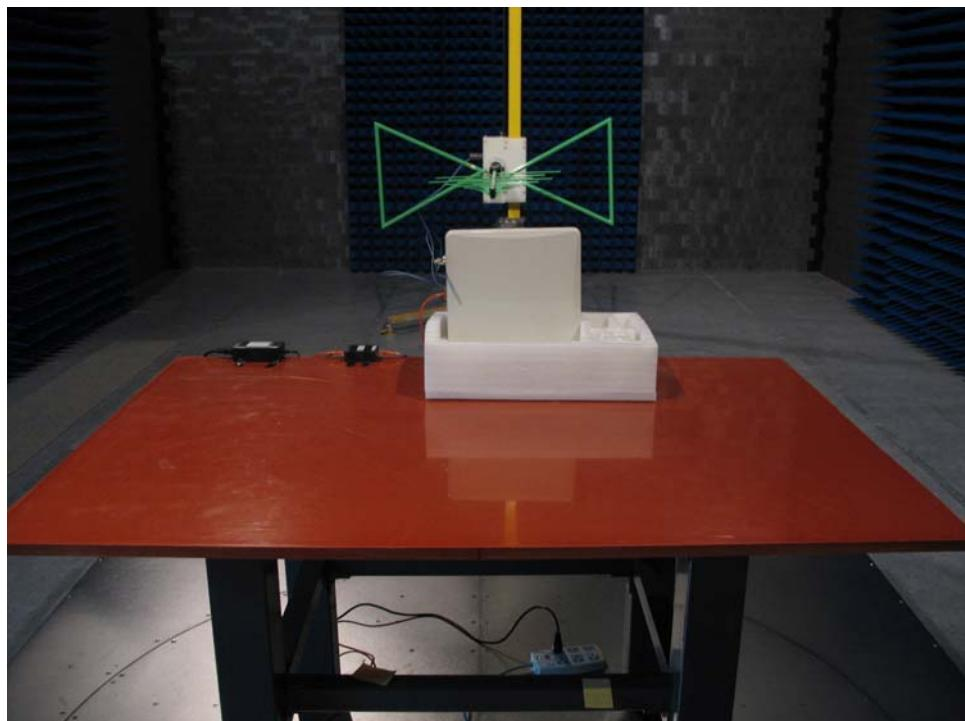
Test Mode: Mode2: Transmitter 802.11g
