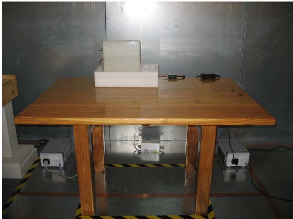
Test Mode : Mode1: Transmitter 802.11b
