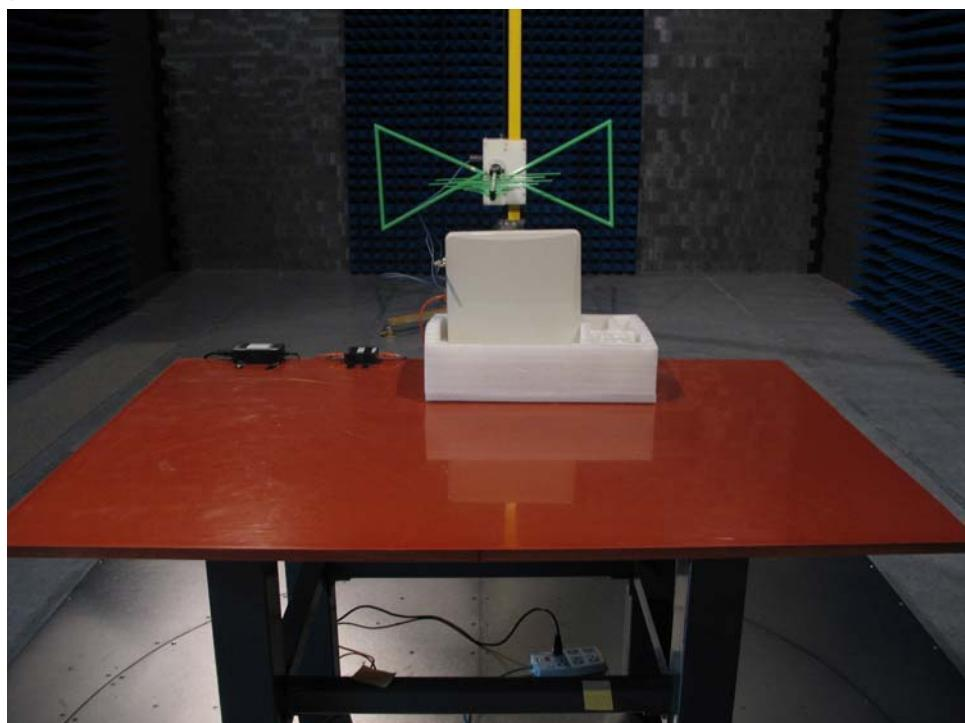
Test Mode: Mode3: Transmitter 802.11a with Outside Antenna
