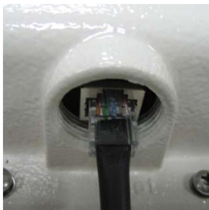
5. Plug water-joint into the Access Point and tighten it.
