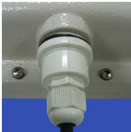
6. Attach the external antenna to Access Point.
