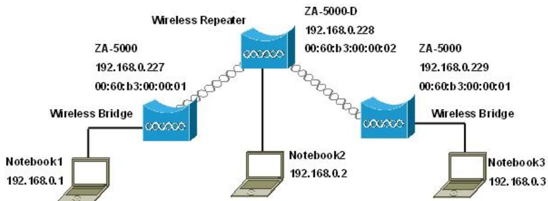
Figure 12 Wireless Repeater Connection
