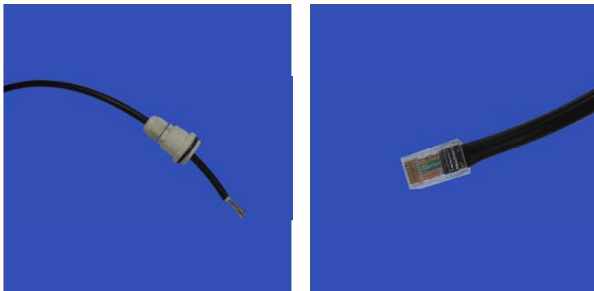
4. Attach STP cable to the RJ-45 connector on the Access Point. Then connect another end of the RJ-45 cable to a hub or a terminal.
