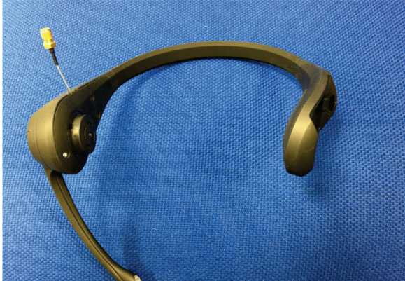
Figure 6: Headset test configuration – cable entry zoom
