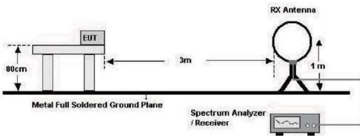
**below 1 GHz (30 MHz to 1 GHz)**
