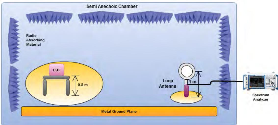
Magnetic field tests shall be performed in the frequency range of 9 kHz to 30 MHz using a calibrated loop antenna.
