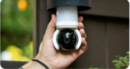
Screw the lightbulb camera into the fixture, making sure it is tightly secured. Do not over-tighten.
