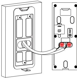
3 Push the wiring through the hole in the wall or door frame. Slide the doorbell down so the **plastic tab on the doorbell** locks into the **notch on the mounting bracket**.
