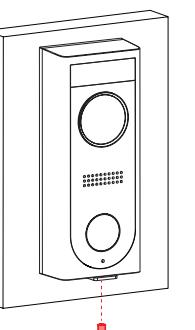
13. Insert the **included security screw** through the mounting bracket and into the screw hole on the bottom of the doorbell. Fasten tightly using the star-shaped end of the included screwdriver to complete the installation.
