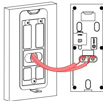
2 Use the **included screws (x2)** to secure the power cables.
