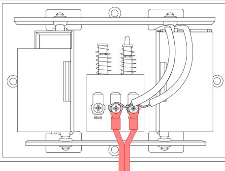
5. Mount the chime kit to the inside of your chime box, or along the cover plate, using the included double-sided tape.
