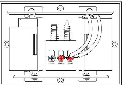
3. Connect the included chime kit to the green terminal on the end of the included wiring as shown below.
