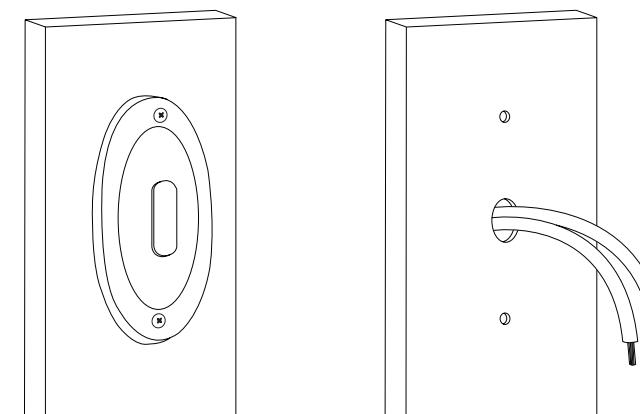
**TIP:** Bend the power cables so they do not fall through the hole in the wall.
