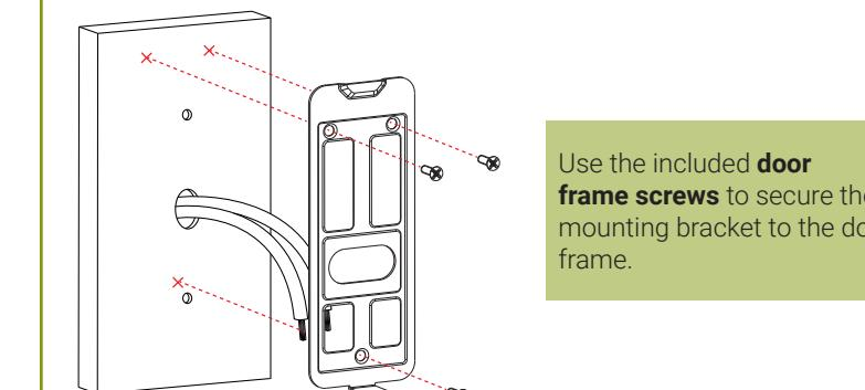
Use the included **door frame screws** to secure the mounting bracket to the door frame.
