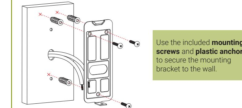
Use the included **mounting screws** and **plastic anchors** to secure the mounting bracket to the wall.
