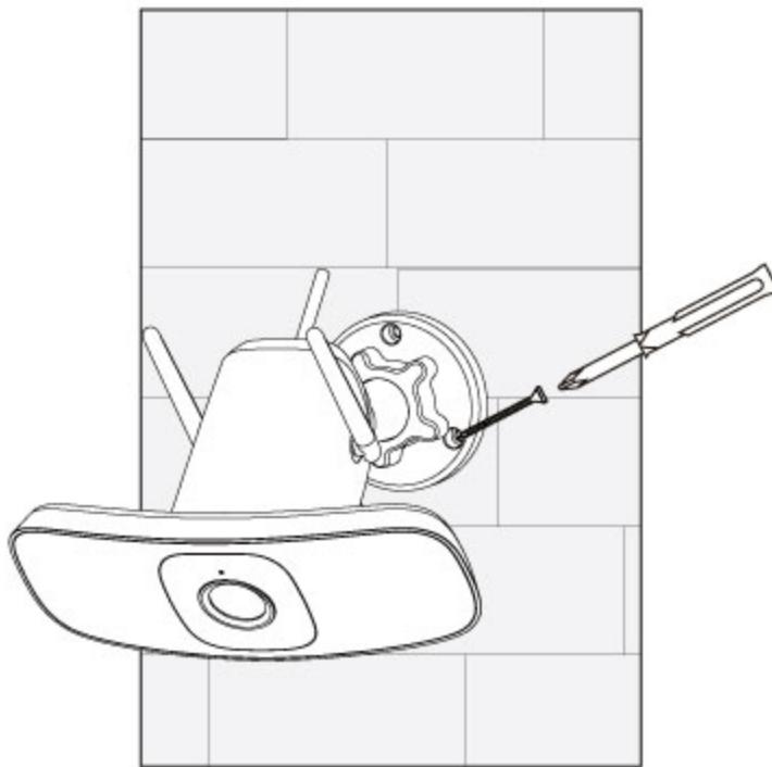
6. Loosen the bracket's adjustment ring by turning it counterclockwise. Position the camera to your desired angle, then tighten the adjustment ring clockwise to lock the position.
