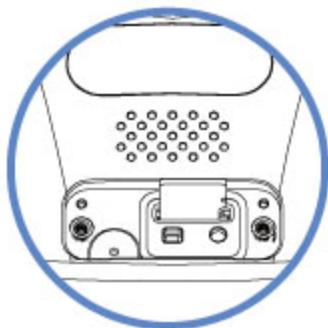
3. Replace the compartment cover and tighten both screws.
