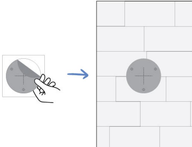
3. Drill where marked. Use drywall anchors if installing into drywall.
