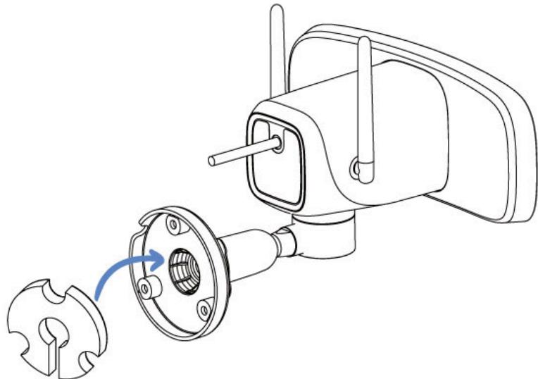
5. Align the bracket over the drilled holes and secure it using the provided screws.
