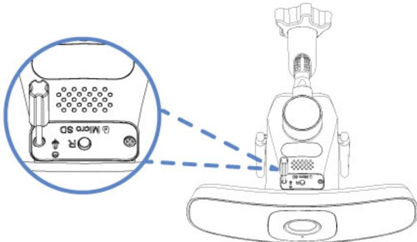
2. Insert a MicroSD card into the slot until it clicks into place.
