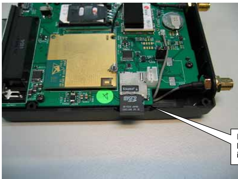
Fig 2.2. MicroSD Card Installation
