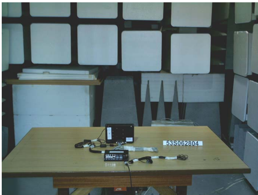
RF Output Power Test Setup (Rear View)
