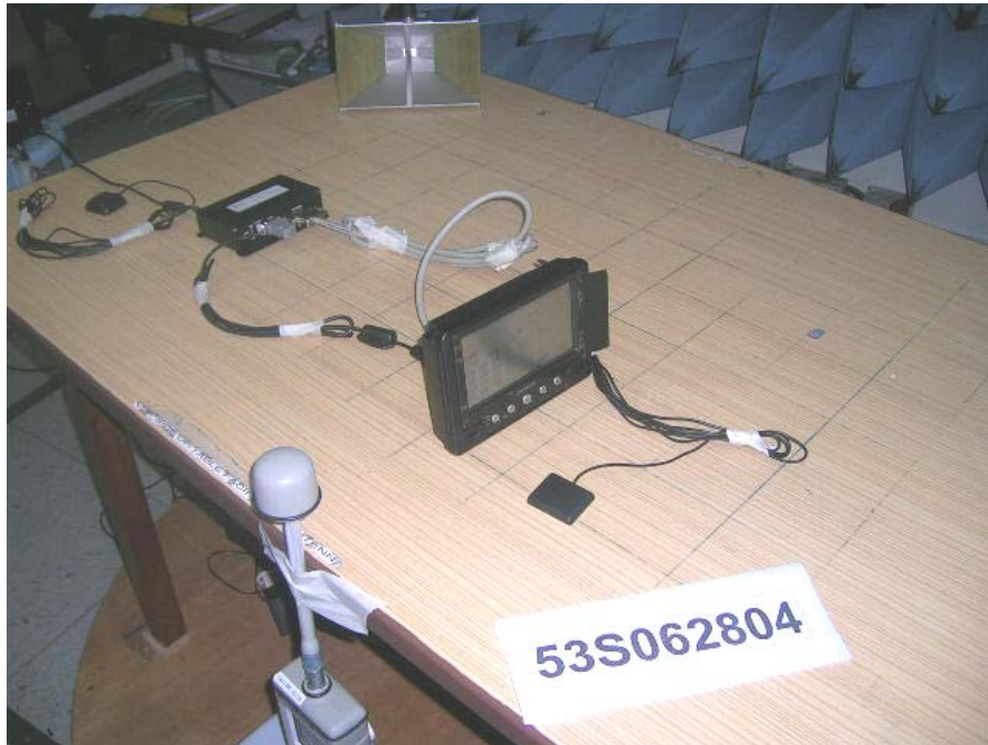
Maximum Permissible Exposure (MPE) Test Setup
