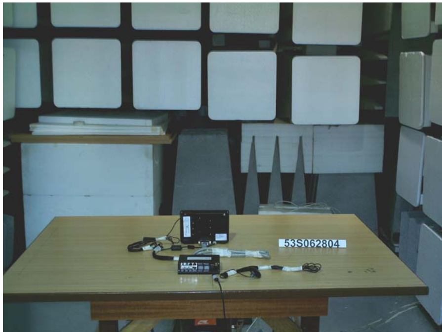
Receiver Spurious Emissions Test Setup (Rear View)
