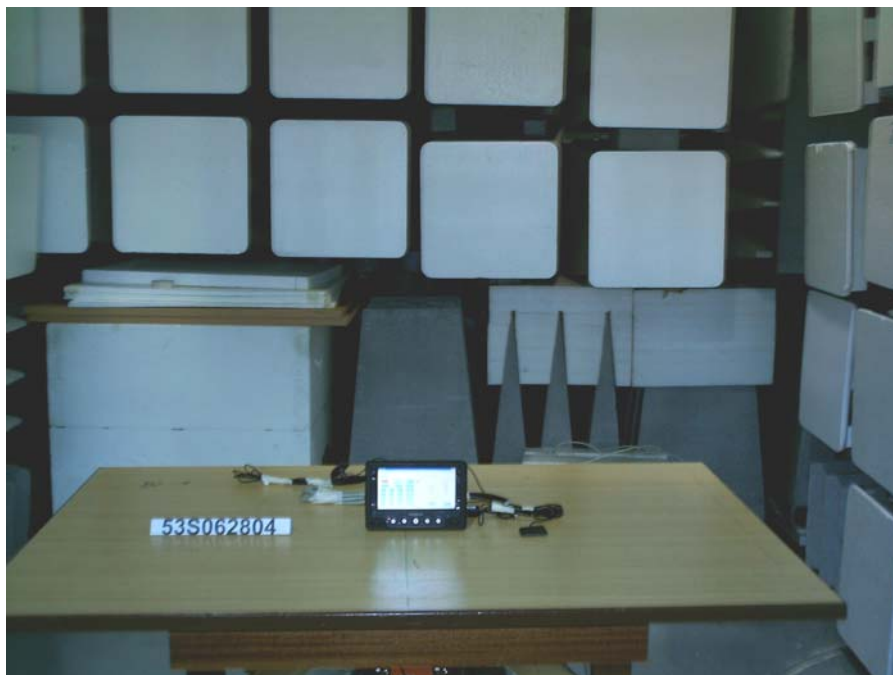
RF Output Power Test Setup (Front View)
