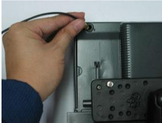
Figure 17 Connecting the GPRS Antenna to the MT Port
