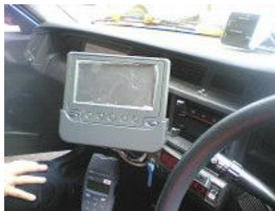
Figure 19 Typical Mounting of MT in the Vehicle- Front View
