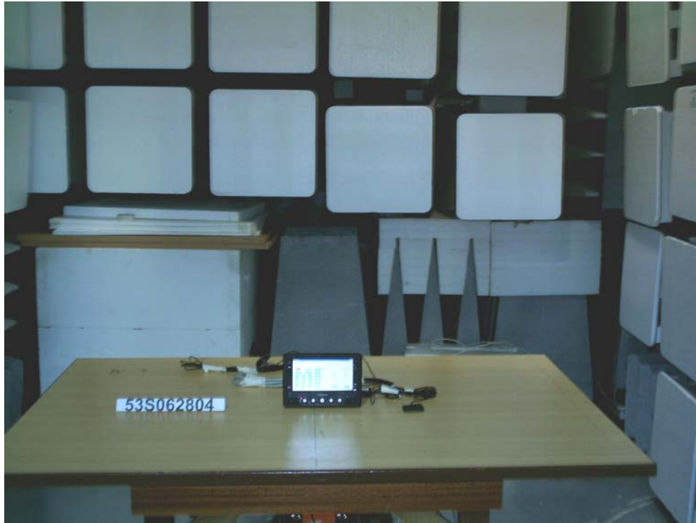
Band Edge Compliance (Radiated) Test Setup (Front View)
