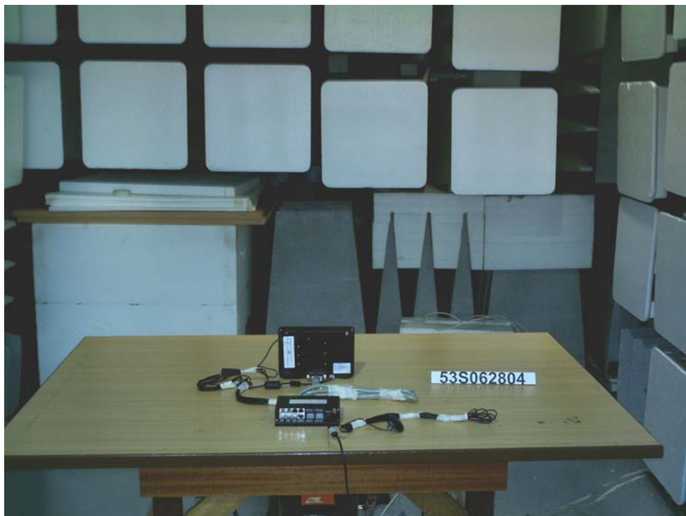
Band Edge Compliance (Radiated) Test Setup (Rear View)
