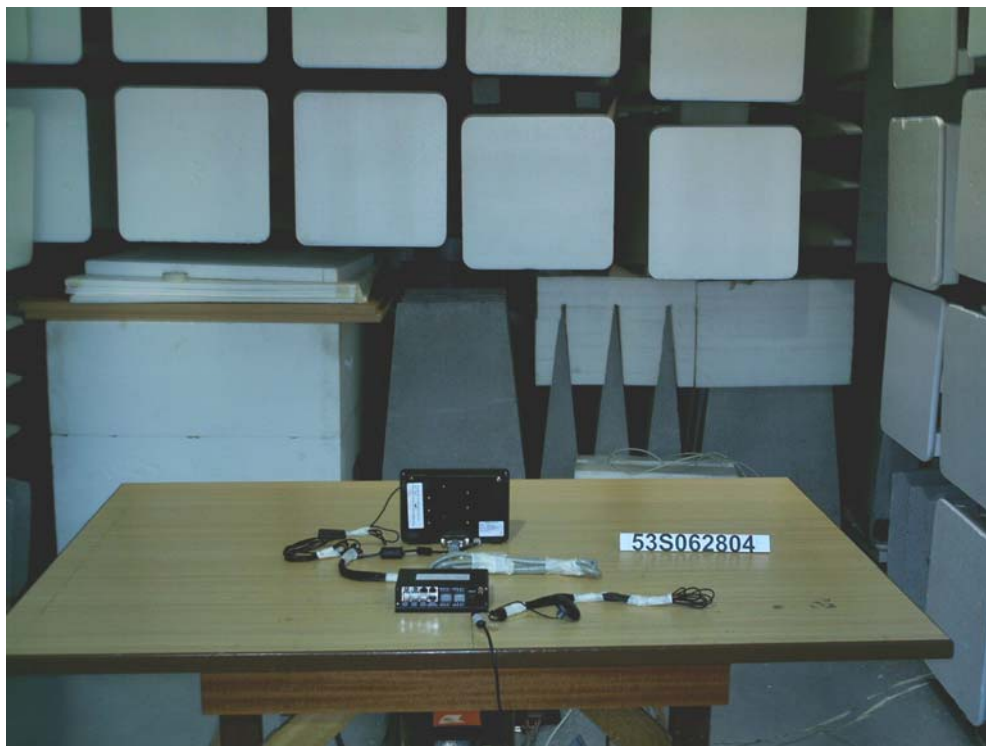
RF Output Power Test Setup (Rear View)
