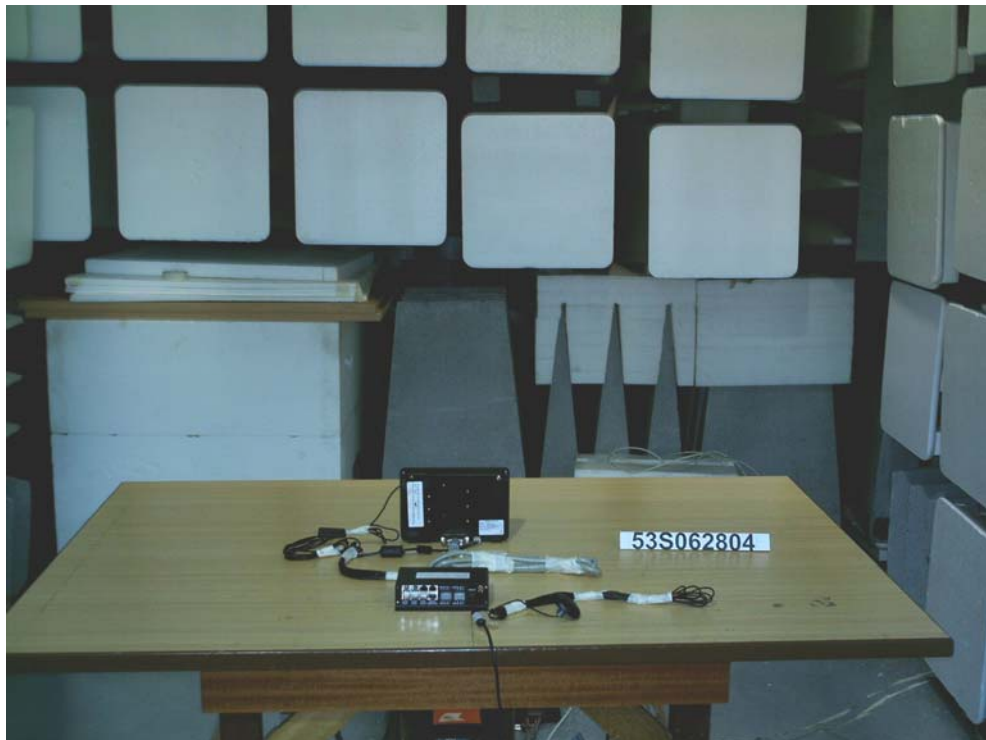
Receiver Spurious Emissions Test Setup (Rear View)
