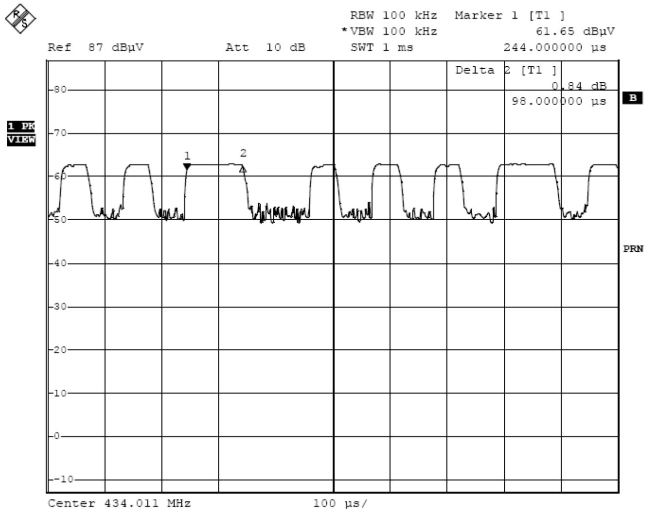
The graph shows the duration of middle 'on' signal. From marker 1 to marker 2, duration is 0.098ms.
