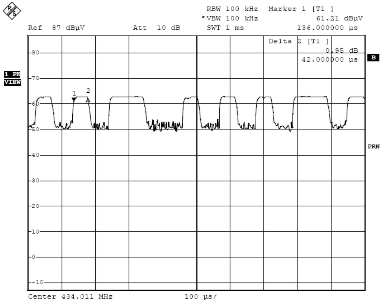
The graph shows the duration of short 'on' signal. From marker 1 to marker 2, duration is 0.042ms.
