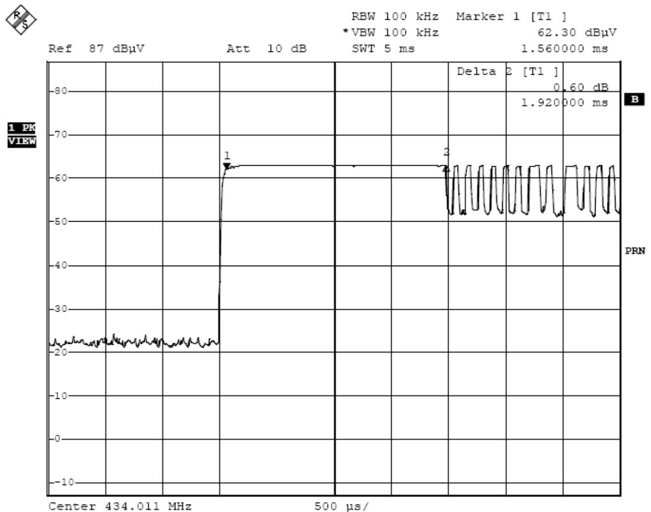
The graph shows the duration of long 'on' signal. From marker 1 to marker 2, duration is 1.92ms.
