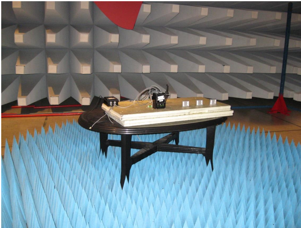
Photo 4.1.3 Test setup regarding measurement of radio frequency electromagnetic field > 1 GHz
