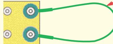
Placing a jumper wire directly across the battery snaps is a **SHORT CIRCUIT**.
