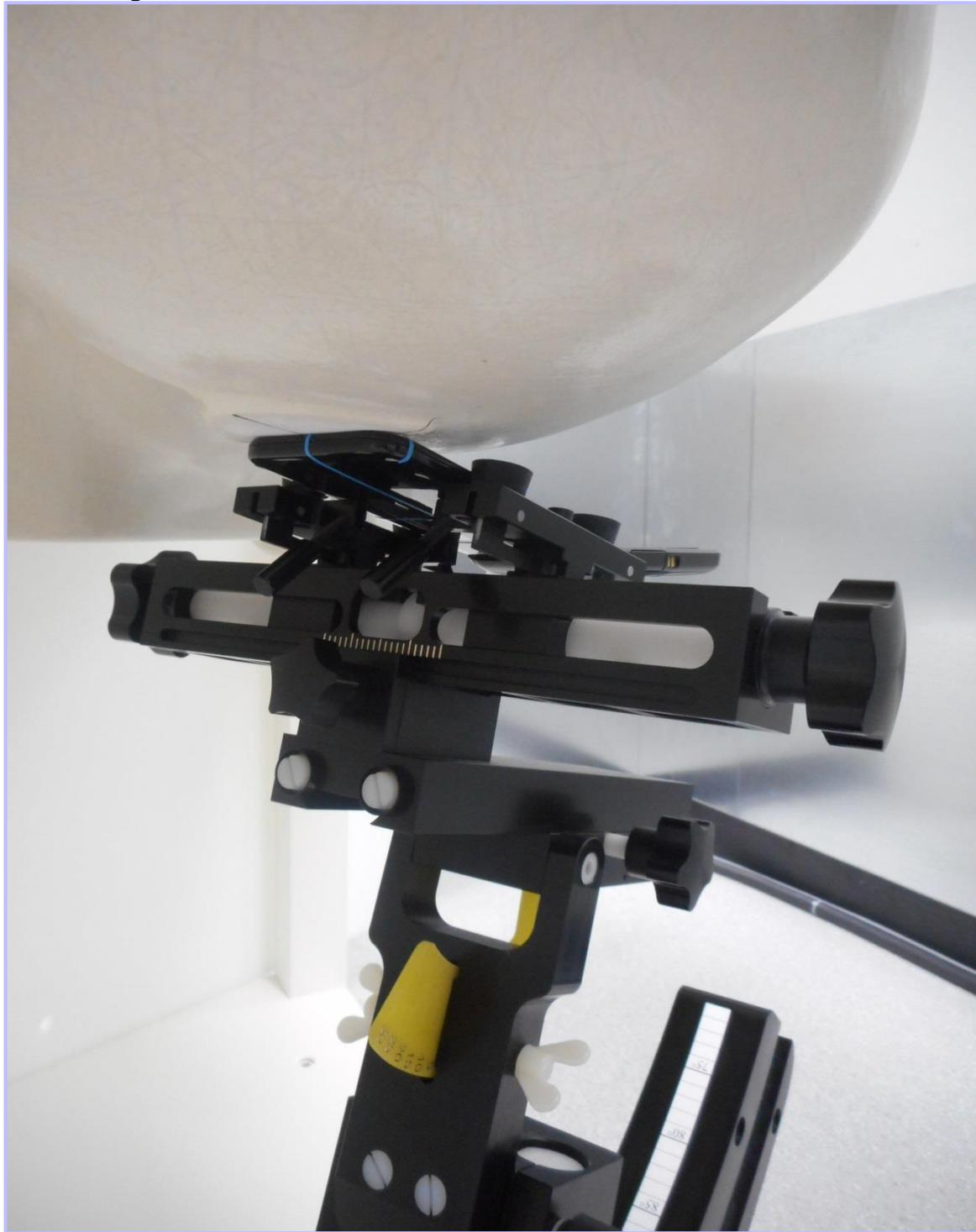
**006: Front Open of EUT at 10mm Facing Phantom**
