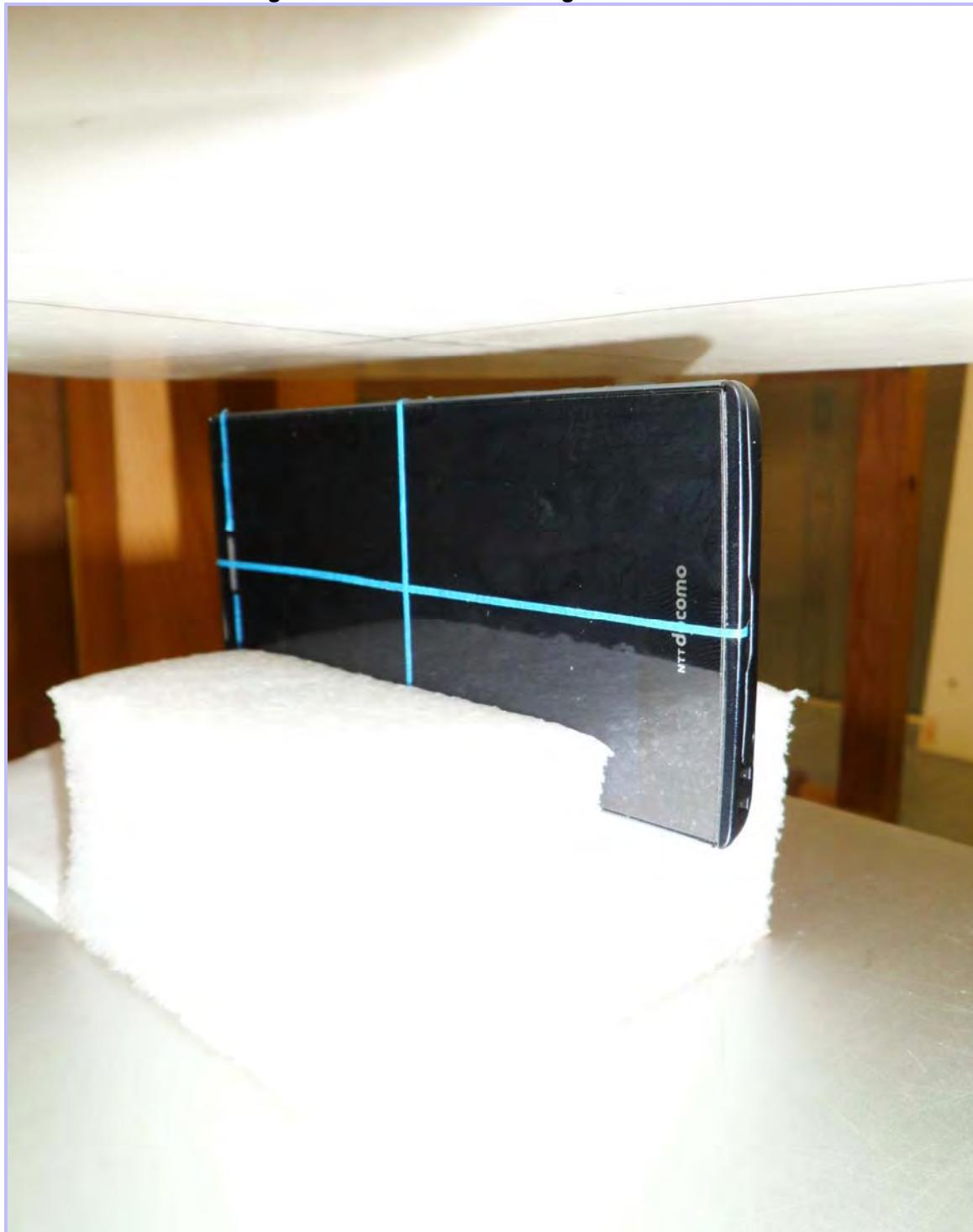
**PHT/87471JD03A/017: Right Hand Side of EUT Facing Phantom With Antenna Extended**
