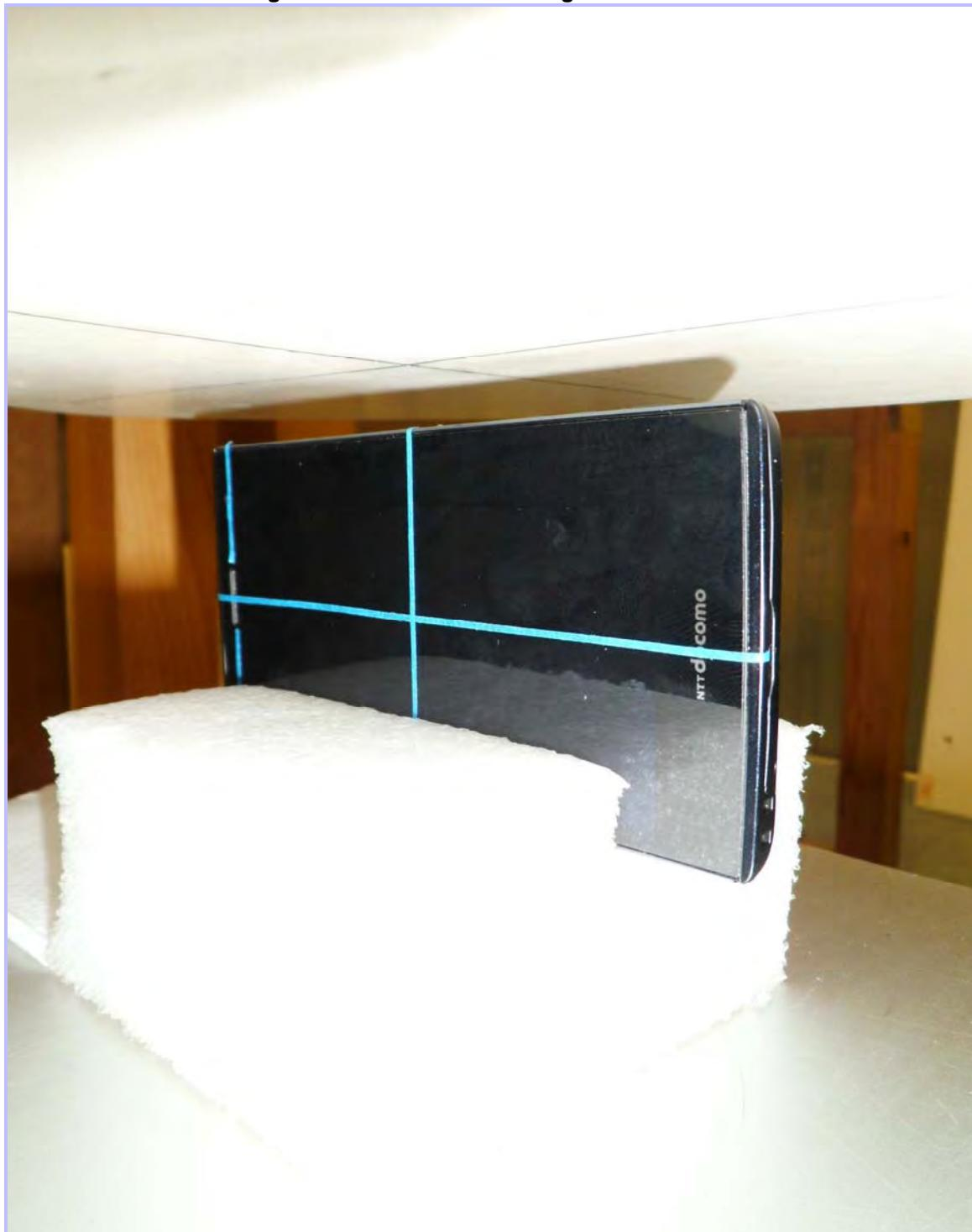
**PHT/87471JD03A/018: Top Of EUT facing phantom Antenna Retracted**
