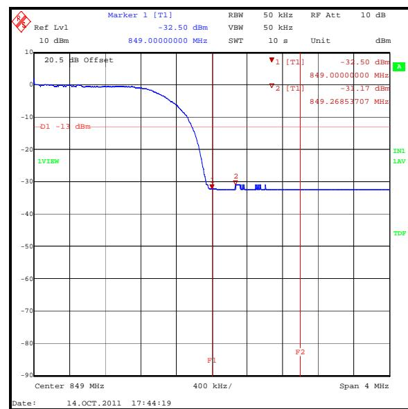
**Transmitter Radiated Emissions at Band Edges (continued)****Results: HSDPA Sub-Test 4**
