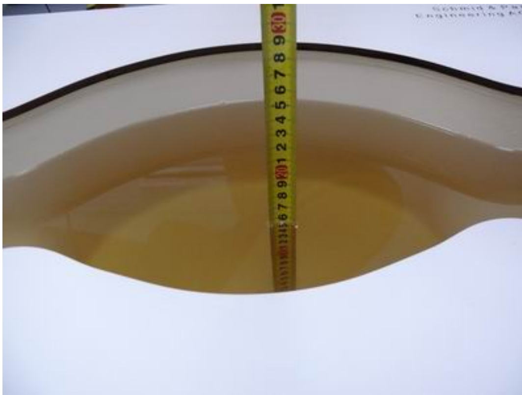
Picture 2: Liquid depth in the flat Phantom (835MHz, 15.4cm depth)
