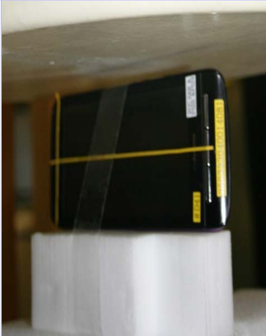
PHT/81533JD05/016: RHS of EUT With Antenna Retracted Facing Phantom
