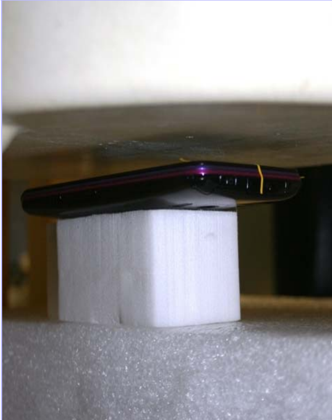
PHT/81533JD05/010: Front of EUT With Antenna Retracted Facing Phantom
