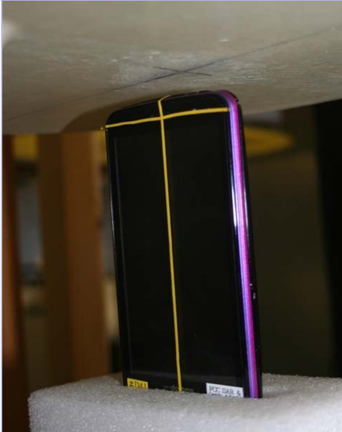
PHT/81533JD05/018: Top of EUT With Antenna Retracted Facing Phantom
