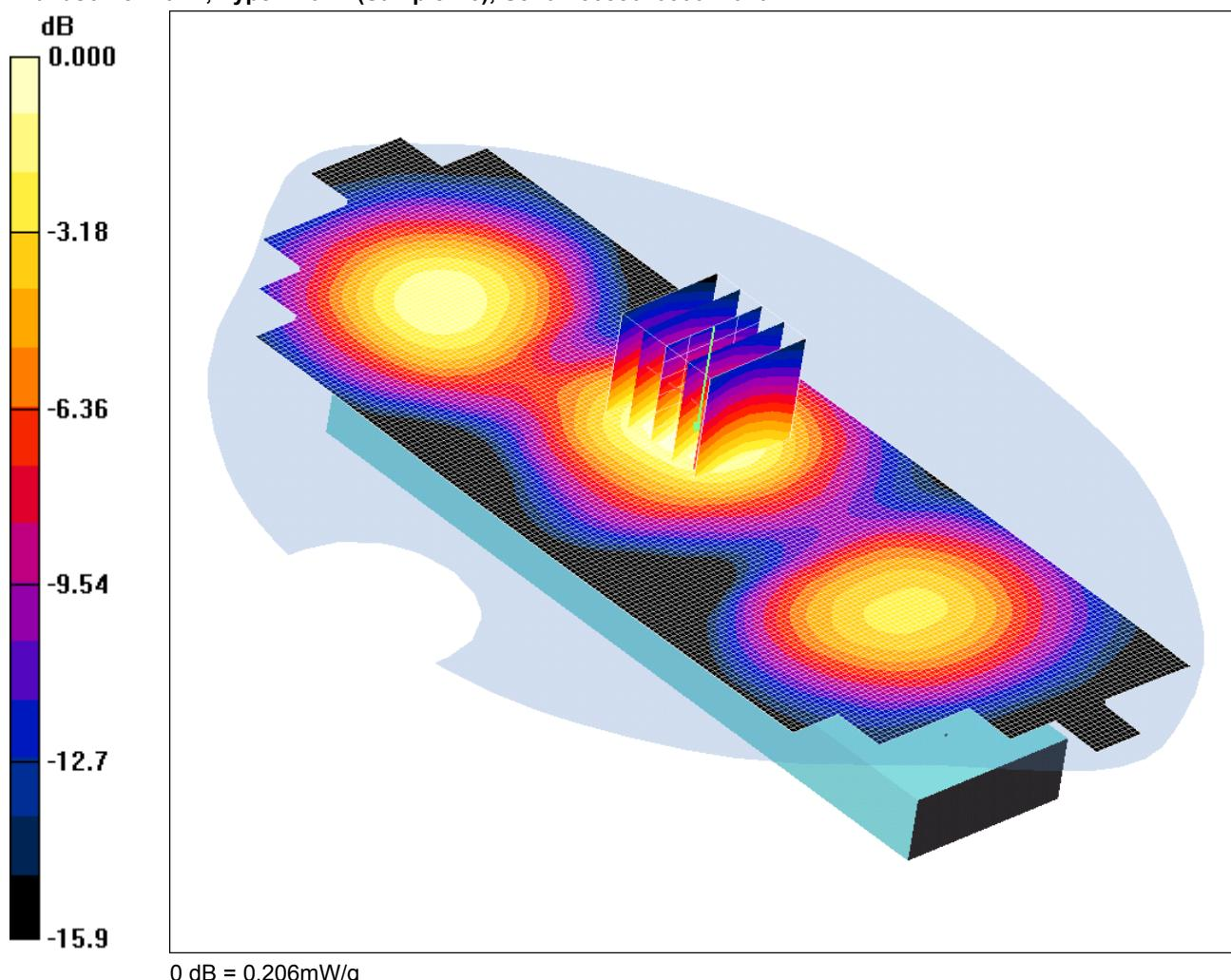
Communication System: GPRS 1900; Frequency: 1879.8 MHz; Duty Cycle: 1:4
