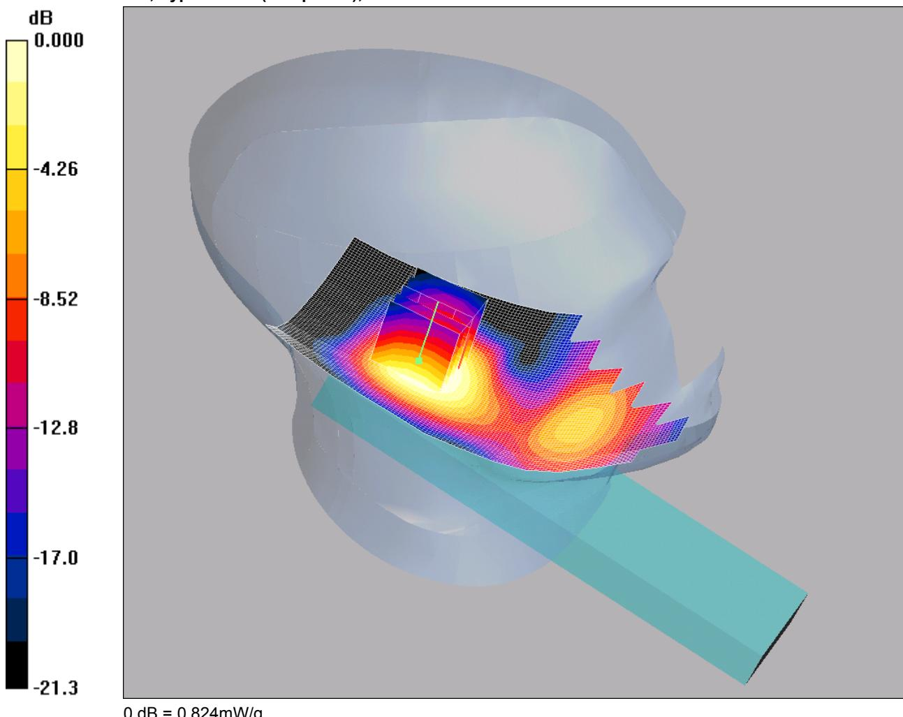
Communication System: PCS 1900; Frequency: 1879.8 MHz; Duty Cycle: 1:8.3
