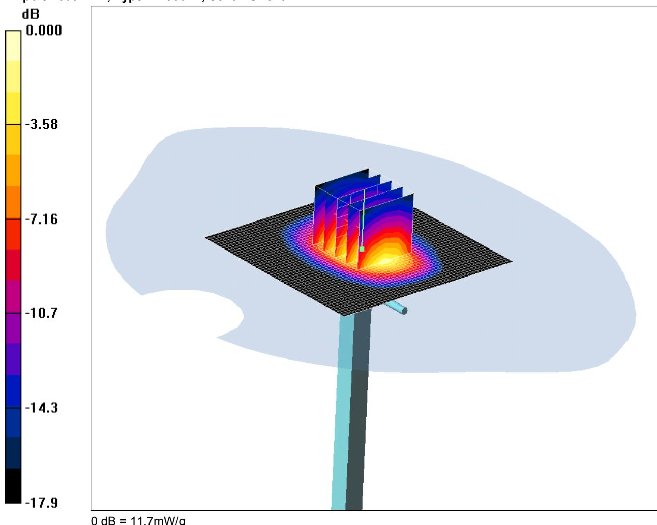
Communication System: CW; Frequency: 1900 MHz; Duty Cycle: 1:1
