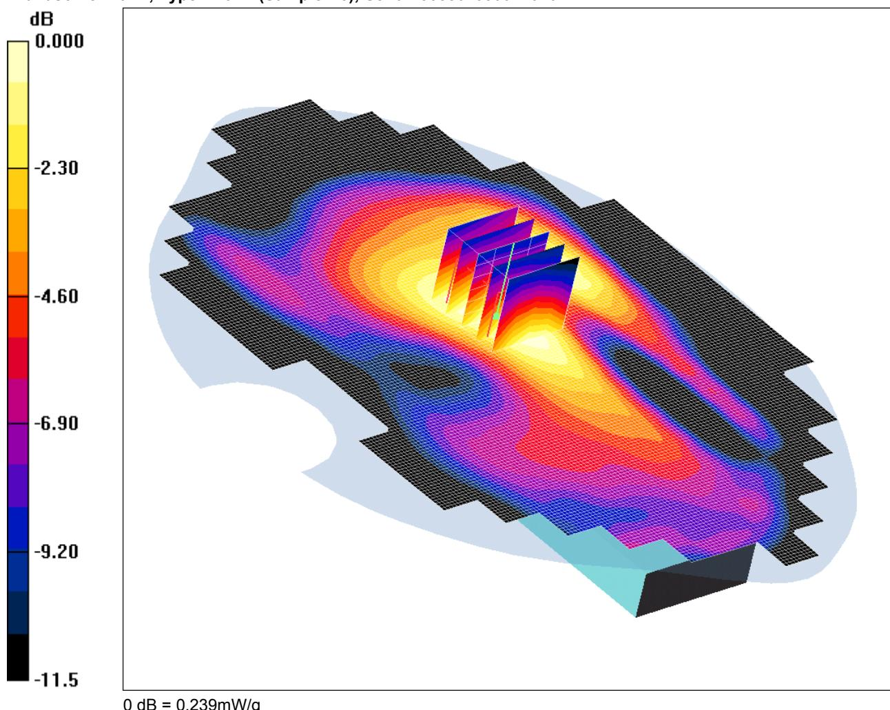
Communication System: UMTS-FDD V; Frequency: 836.6 MHz; Duty Cycle: 1:1
