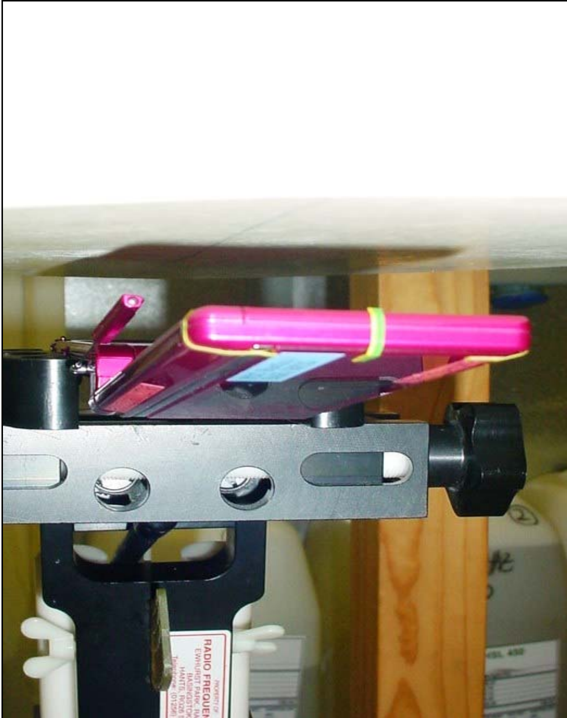
PHT/75983JD07/015: Front of EUT with Antenna Extended Facing Phantom at 15mm
