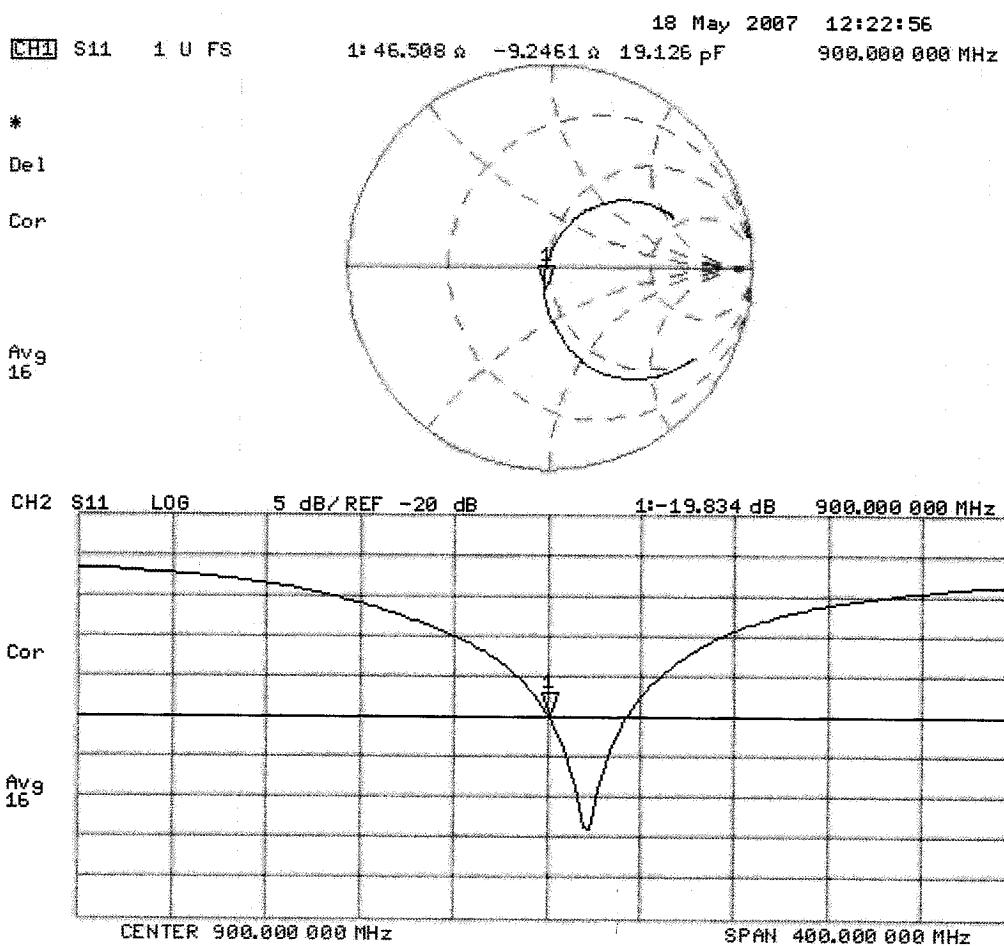
**Test of: NTT docomo P-07A****To: OET Bulletin 65 Supplement C: (2001-01)**
