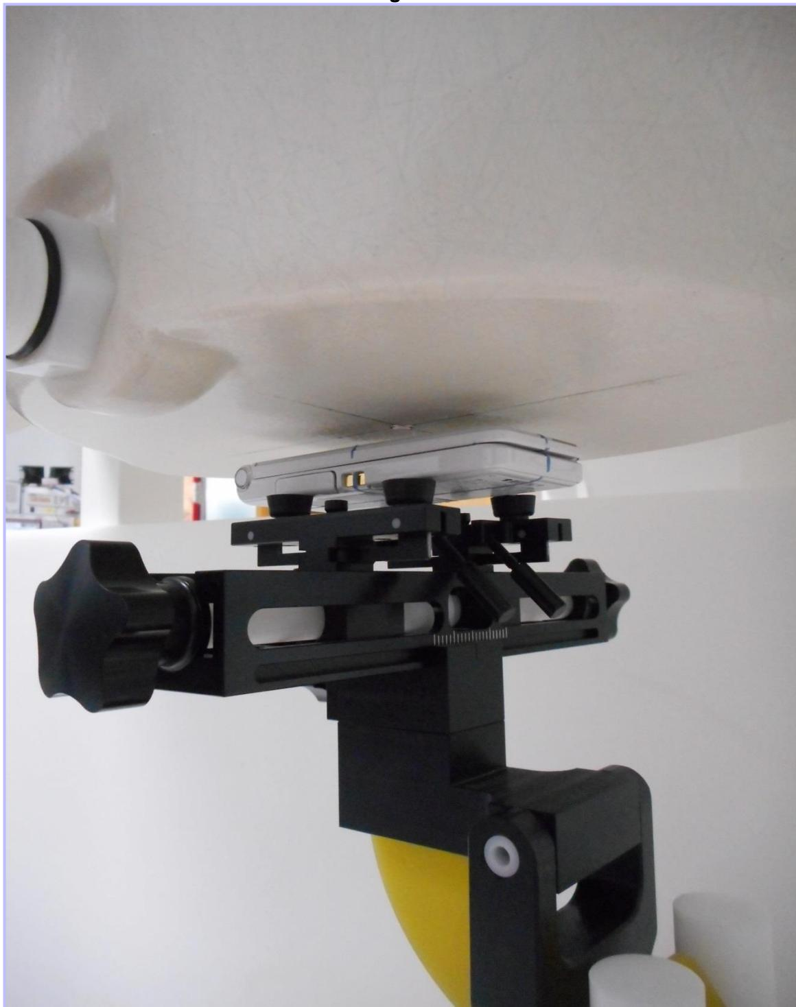
**007: Back of EUT Closed at 15mm Facing Phantom**
