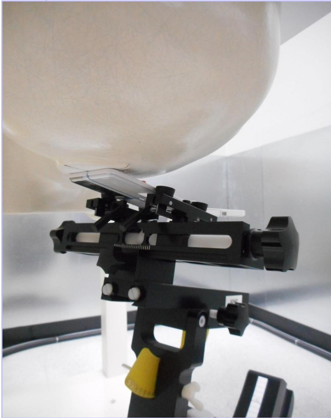
**006: Front of EUT Closed at 15mm Facing Phantom**
