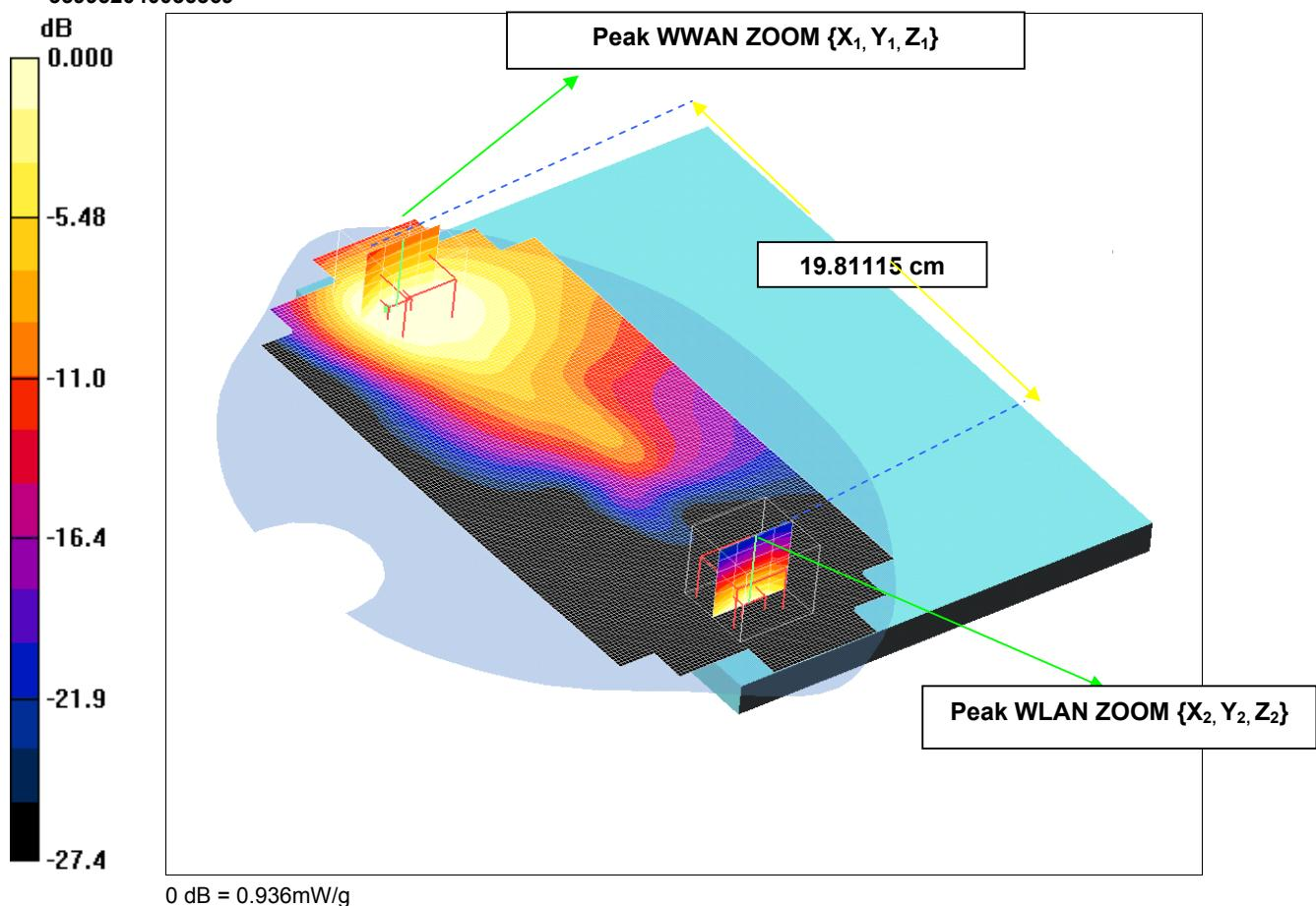
Note: The above SPLSR calculation is only presented for worst case SAR measure on WWAN (Base of EUT with Antenna Retracted facing Phantom UMTS FDD V CH4233) and WLAN (Base of EUT with Antenna Retracted facing WLAN 802.11b 1Mbps CH1). The complete list of all possible SPLSR is given in section 7.2.3.
