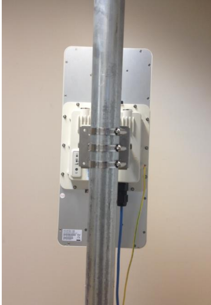
Figure 17 - Typical setup of A3-Ei on the pole
