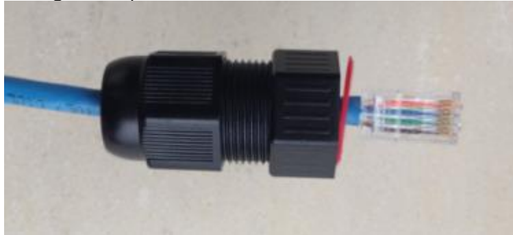
Figure 11 - Use the crimping tool to crimp the RJ-45 connector to the Ethernet cable
