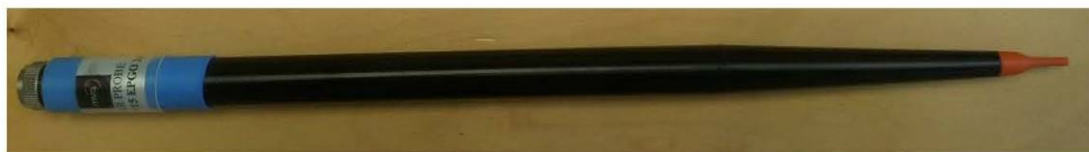
Figure 1 – MVG COMOSAR Dosimetric E field Dipole
