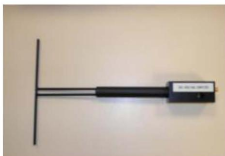
Figure 1 – Satimo COMOSAR Validation Dipole
