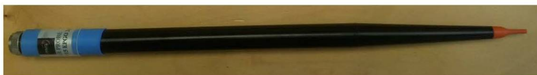
Figure 1 – MVG COMOSAR Dosimetric E field Dipole
