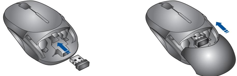
**English** **To readily carry the mouse:** (a) Open the battery case. (b) Insert nano wireless receiver inside the compartment by the direction of the arrow. (c) Close the battery case back.
