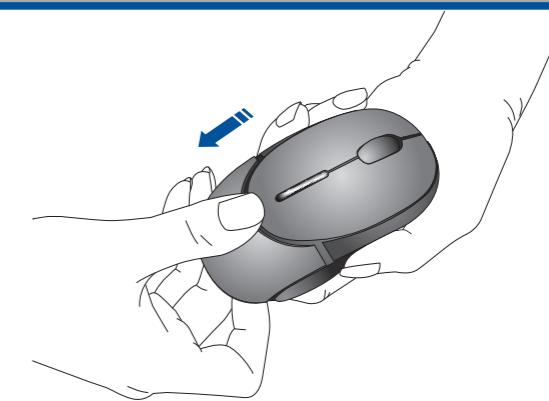
**English** At the bottom of the mouse, follow the direction of the arrow to push gently, at the same time, to pull out the battery cover in opposite direction, to pull out the battery cover.
