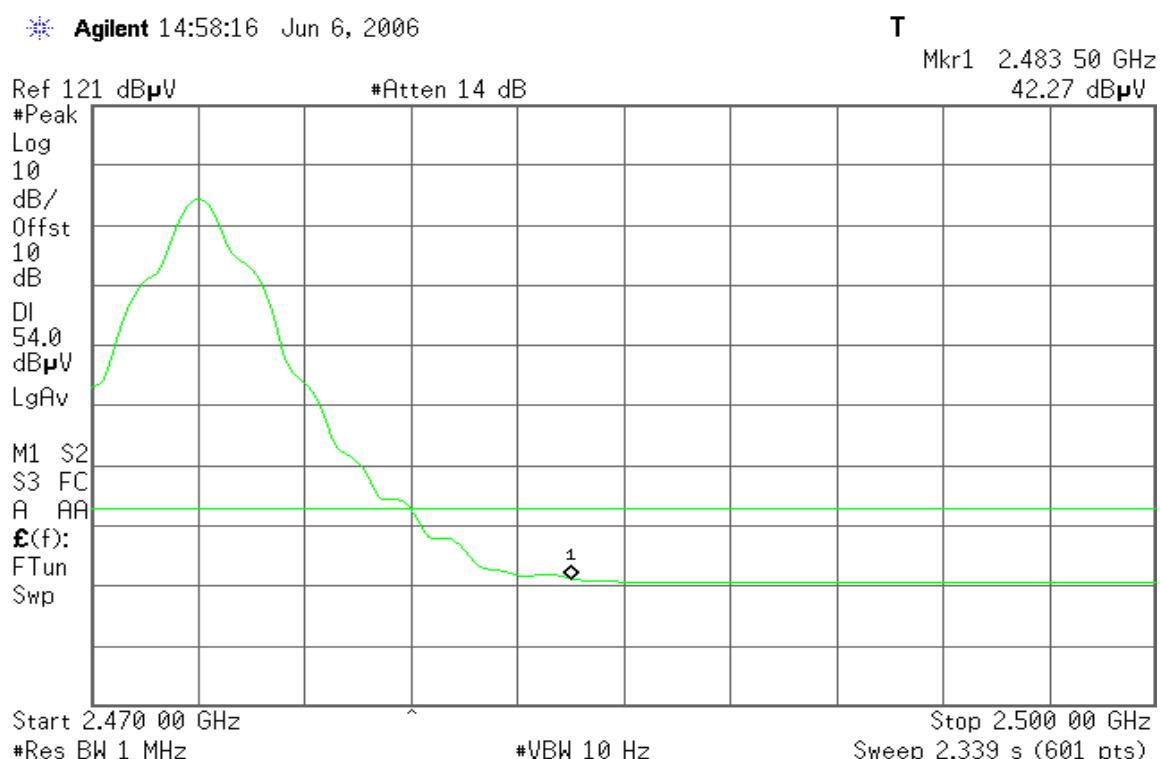
**Detector mode: Peak****Polarity: Horizontal**
