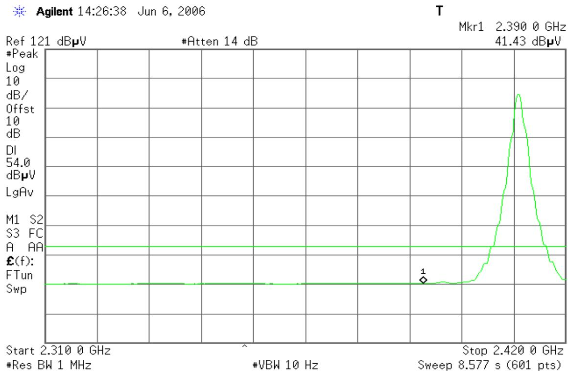
**Band Edges (CH High)****Detector mode: Peak****Polarity: Vertical**
